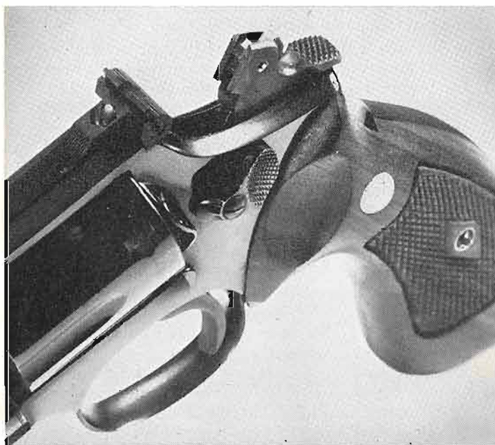
Details of lever-knob that changes the position of striker, changes firing from rimfire to centerfire.
