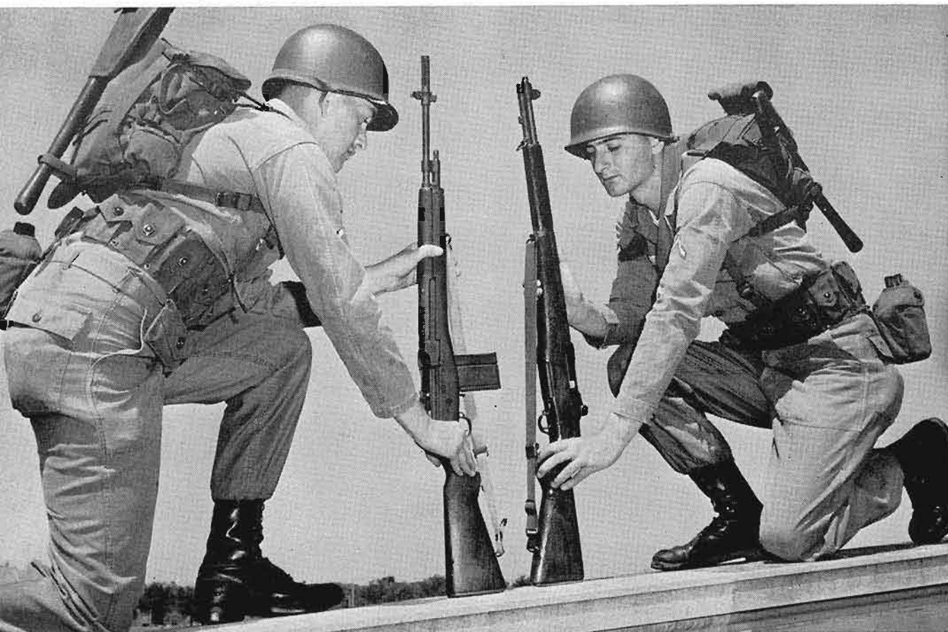
Light rifle program to replace bulky M-1 (right) with lighter, shorter new gun culminated in M-14 (left), formerly called T-44, and is inches longer, half pound heavier.
