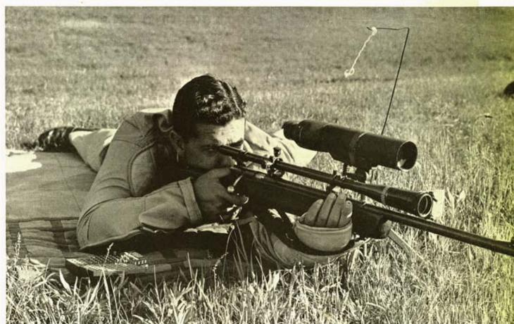
Because basic design of Mossberg .22 single shot was not adapted to reliable machine rest testing, accuracy firing was done with 20X scope fitted, and under careful range conditions to insure maximum, reliable performance of gun.
