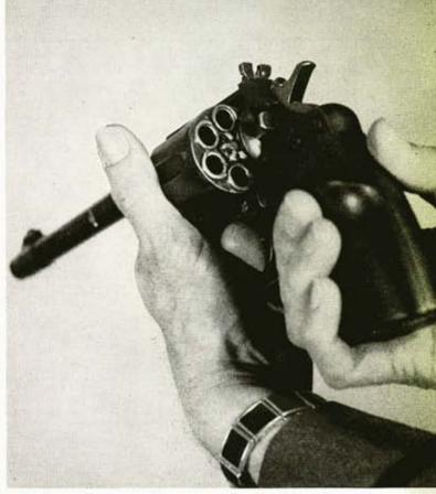
Chambers of .45 revolver were lined with tool steel bushings counterbored to recess case heads and then pressed in, which adapted gun to smaller cartridge.
