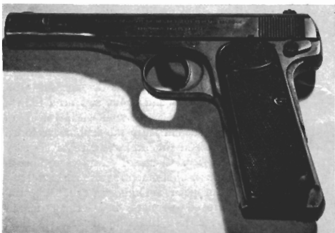
Reliable Browning Model 1922 automatic pistol in .32 caliber was designed by maker especially for police.
