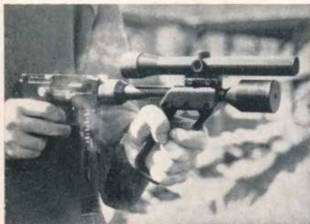
The Seggern .22 SMG prototype with the semi-auto trigger assembly and 20-round clip scoped by a Bushnell.
