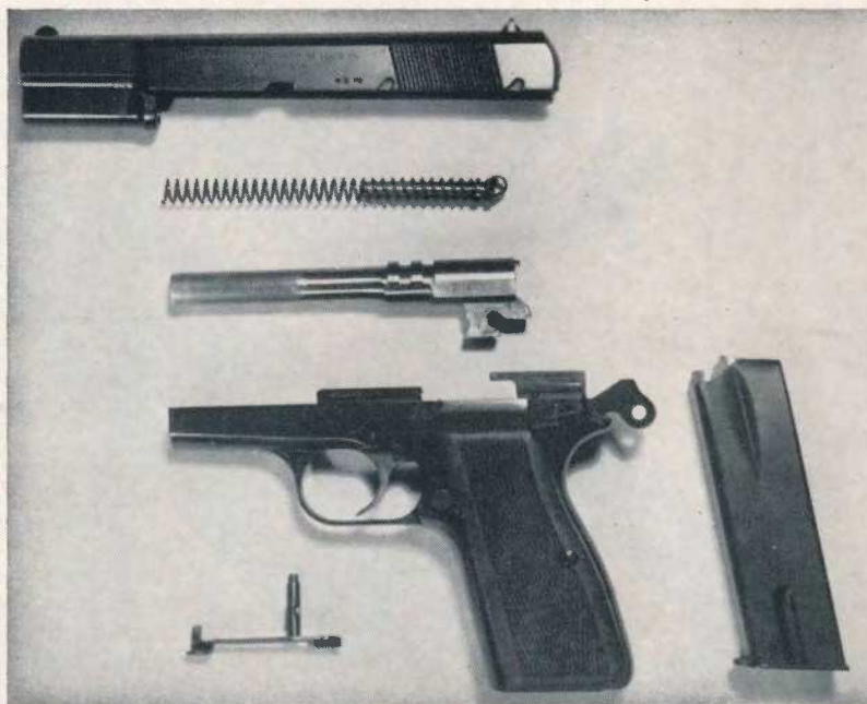
A stripped Hi-Power shows a fixed bushing on the slide, a fixed cam lug on the barrel and the big 13 shot clip.
