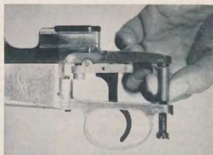
Position of guard screw bushing.
