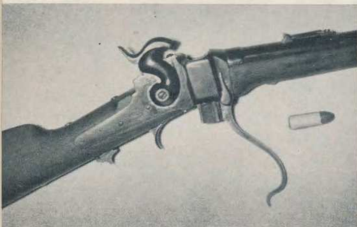
The breechloading Sharps percussion carbine quickly became the Indians' favorite rifle.
