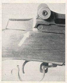
Receiver needs a clearance forward of rear curve. On handguard ends, leave 1/32" for heat to expand.
