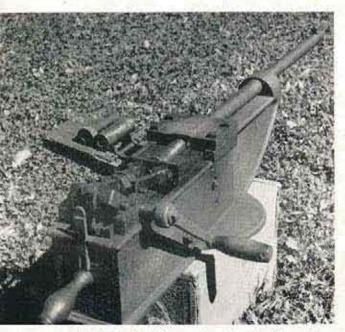
Shells in feed tray roll onto spindle, putting each shot in line with the moving breech bolt.
