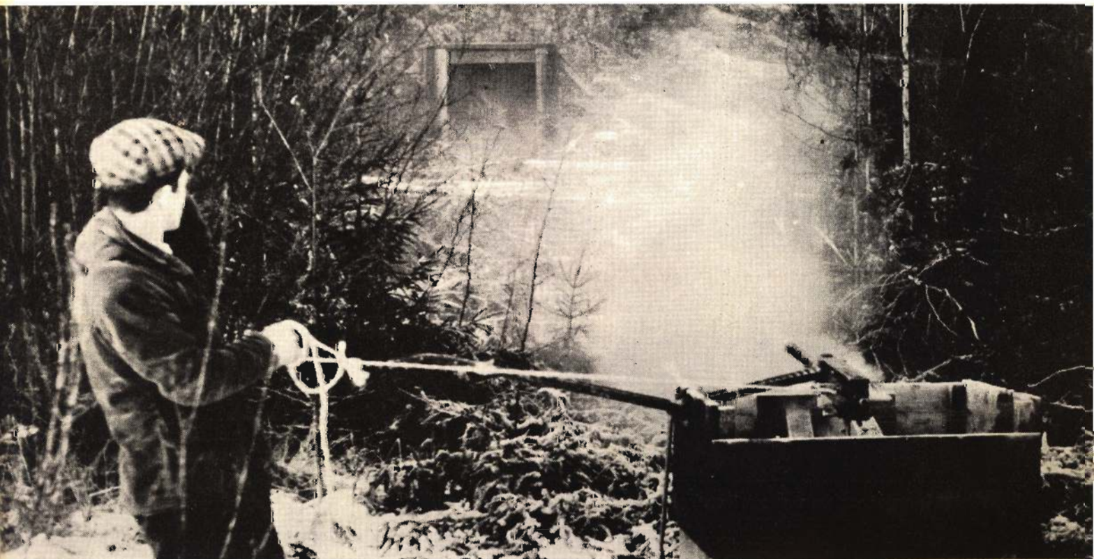
Fully-automatic bullet making and case sizing machines at Norma (above) chomp out loaded ammo and components which must be mass-tested to save time. Below, air-cooled Browning rips out string of reloaded .30 brass in case endurance test.
