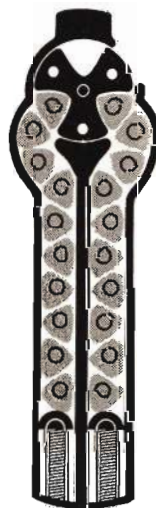
Handful of Fortiflex cartridges called "trounds" because of unique shape stack into magazine in rows as shown by diagram of Dardick open-chamber firearm.
