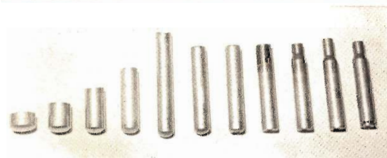
Norma is major custom ammo maker. Top photo shows five of Weatherby Magnum lineup, then 7&61 Sharpe & Hart, and Jap 7.7 and 6.5 dimensioned from sample rifle chambers. Cases are punched in stages from cupped blanks of brass.
