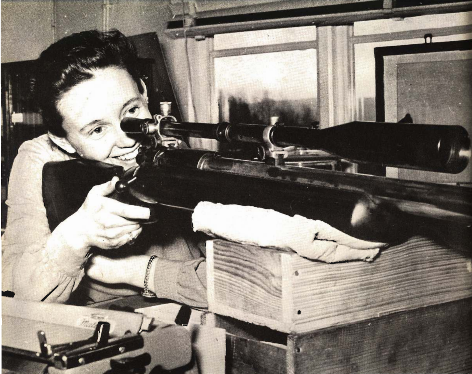
Norma bullets are tested in bench rest outfits such as this heavy Hopkins & Allen U.S.-made Mauser being fired by comely Swedish ballistic lab technician.
