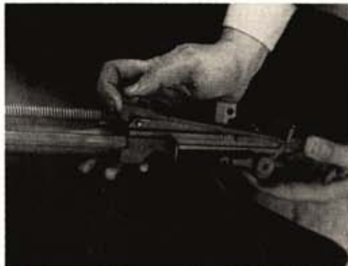
Fire control lever and switch (receiver right rear) can be dismounted easily; receiver is much simpler than M1's. Gas cylinder group (above, right) uses expanding gas to work the action. Action, bolt, operating rod (below) are shorter than M1.
