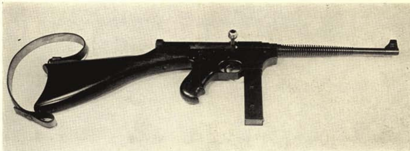
Prototype Neuhausen SIG machine pistol (M1941) resembles American Thompson slightly, was never mass-produced. Swiss encourage automatic gun designing.
