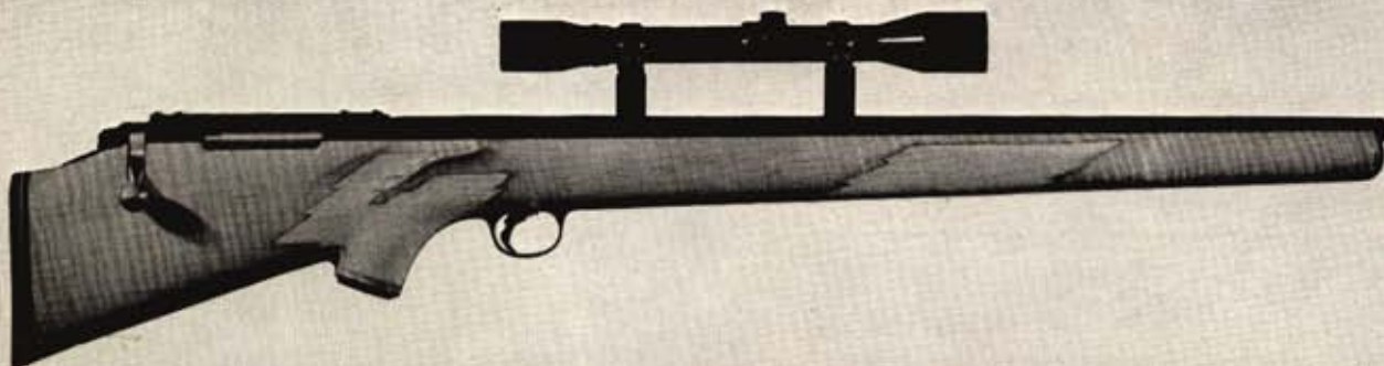
Flashy-stocked bullpup in maple by Lenard Brownell uses Remington 721 action, long barrel, to get top accuracy from rest for varmint and target shooting. Breech has shield.
