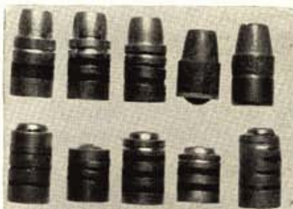
Bullets for .38 Spl. handloads are (top) H & G 51; Ideal 357446 & 358156; and two Harveys. Bottom are Ideal 358432 & 358424; H & G 50 & 41; and defective cast slug from "custom" load.
