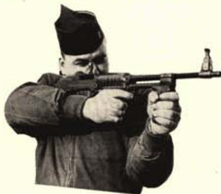
Bull pup version based on BAR was developed by W/O Loren C. Cook.
