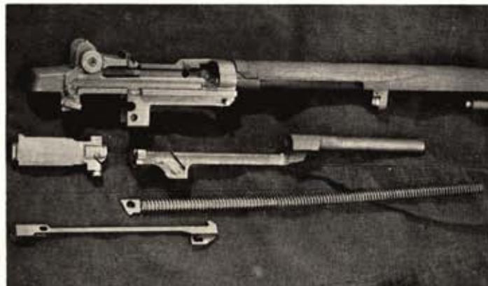
Fire control lever and switch (receiver right rear) can be dismounted easily; receiver is much simpler than M1's. Gas cylinder group (above, right) uses expanding gas to work the action. Action, bolt, operating rod (below) are shorter than M1.
