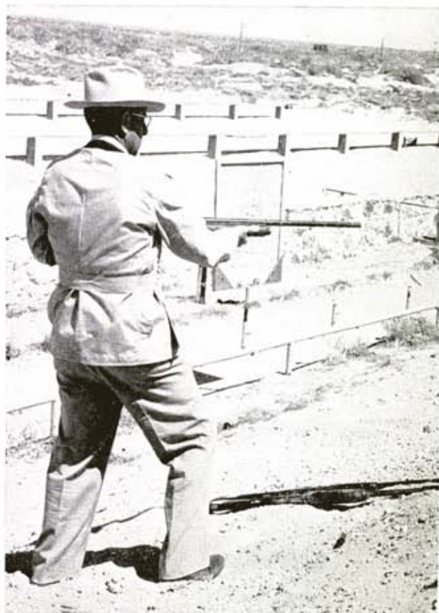
Unlike some recoil-operated guns, gas operated M58 will shoot okay even if not solidly held against shoulder.
