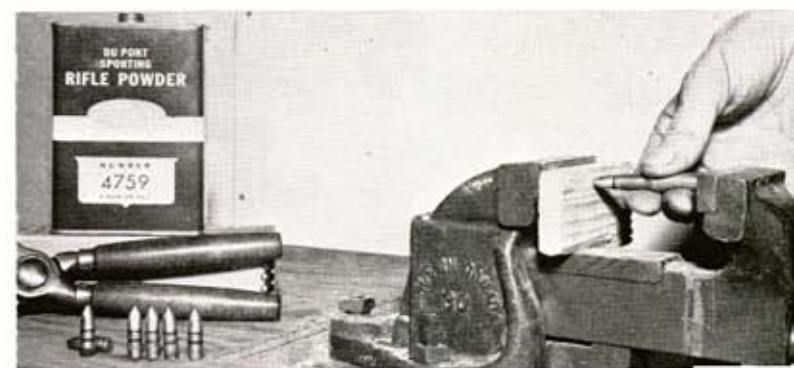
Common vise doubles in brass as bullet seater using soft wood to cushion lead bullet tips from denting.
