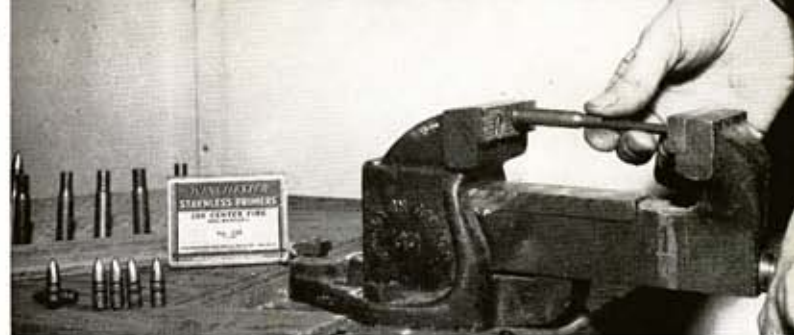
Case swollen to fit rifle chamber exactly by first firing is capped using steel rod and vise for pressure.
