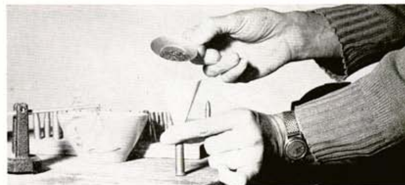
Charge should be weighed for accuracy but old case sawed off to hold right amount of powder is good measure.
