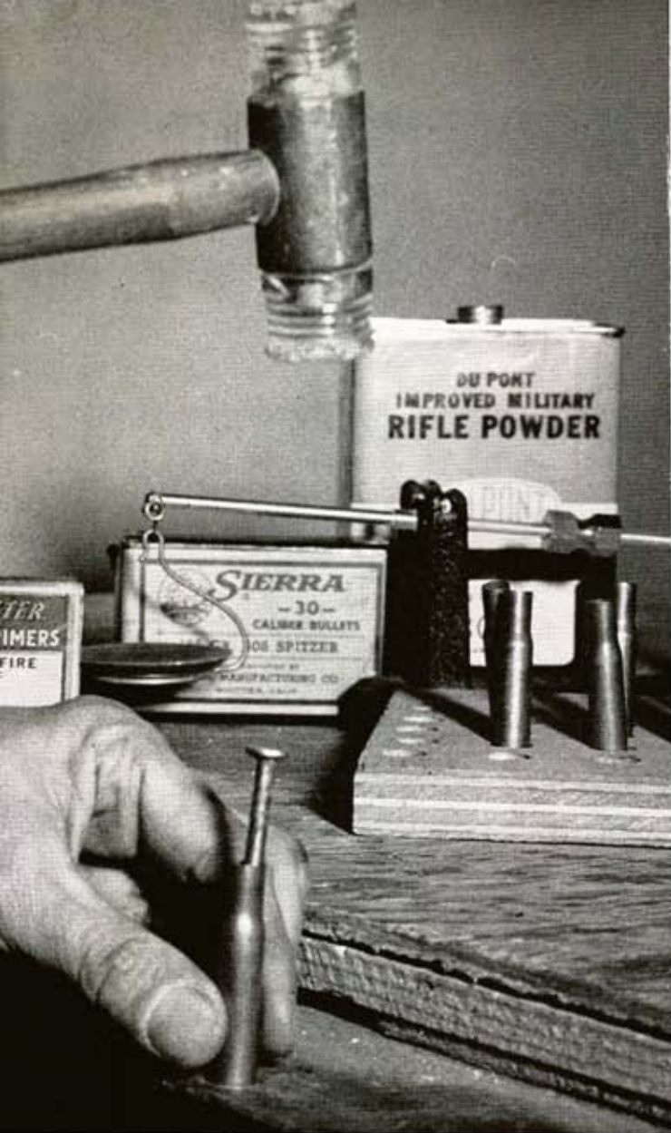
Rough and ready decapping punch from old nail is first step in cooking up precision fodder to accurize .30-30.
