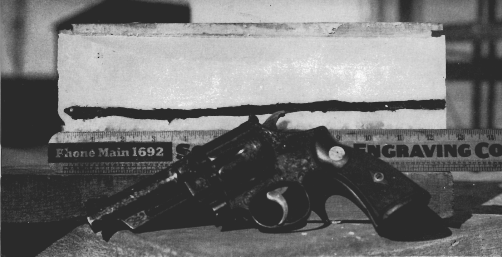
Magnum loaded to original prewar velocity penetrated 12 \frac{3}{4} inches in solid block of paraffin. Gun does not have that powerful wallop today since manufacturer has reduced load about 10 per cent as indicated in recent tests.
