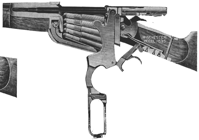
Browning's later Model 95 for Winchester had box magazine for pointed bullets, was chambered for hot .30's. Both rifles used sliding breech blocks, rear locked.
