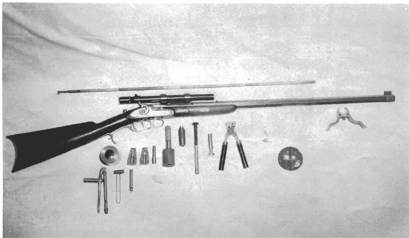
Seth Millard .35 caliber rifle used by Captain Elliott was handmade by master New York gunmaker. Accessories include four parts of the bullet swage and an unusual detachable muzzle rest. Front trigger breaks gun for loading.
