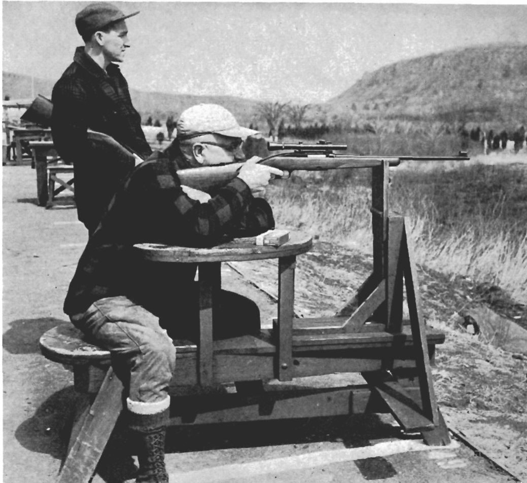
Firing the Model 88 Winchester from a bench rest with scope revealed that groups of about 3" at 100 yards were ordinary in this light lever rifle.
