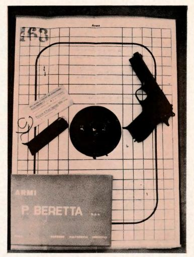
From the Beretta factory comes a test target, the Brigadier pistol, a spare magazine, proof firing tag, and container.
