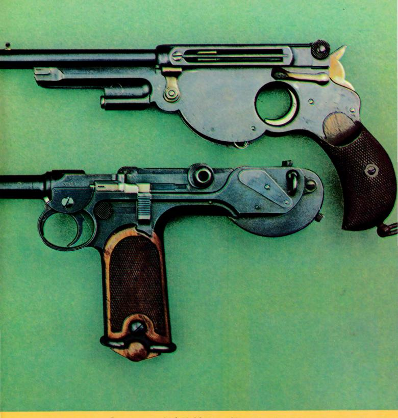
Bergman auto pistol, Model 1894, caliber 7.65, 5-shot. Below is the first of the semiautomatic pistols, invented by Hugo Borchardt, and made by Lowe of Berlin. These guns, serial nos. 5294 and 5286, from the collection of Musee d'Armes, Liege.
