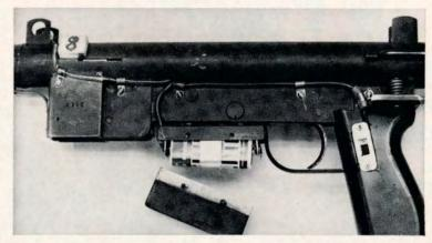
Smith and Wesson's M76 submachine gun, modified for experimental caseless ammunition, uses electrical ignition system.
