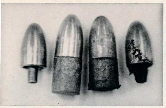
Bullet with anchor nubbin; normal round; after chambering; heat tested.
