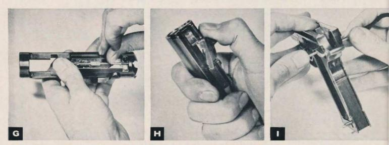
Make sure the smooth side of the indicator pin is up (G) when inserting it. The locking block will snap into place under thumb pressure (H). The sear and ejector are aligned with the hammer strut (I) as the sear pin is inserted.
