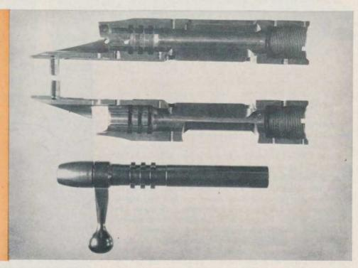
The receiver of this Remington 788 has been cut in half to show the location of the lug recesses. Note that the metal is quite thick in the lockup area.
