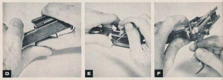
The slide cover is removed through pressure of the magazine follower tool (D). The extractor is snapped out of the frame (E) with hammer strut. The hammer and associated parts are aligned for assembly with hammer strut (F).
