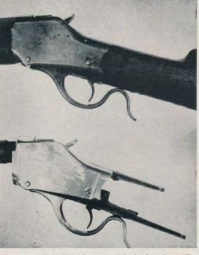
Top: Winchester with thick side walls. Bottom: Side walls were soon milled.
