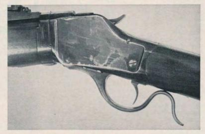
An interrupted thread take-down system was used on some of the Winchester High Walls as well as some of the Low Wall version.
