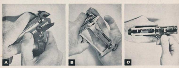
The toolless stripping job begins by using the safety to release the magazine's floor plate lock (A). Removing the magazine catch (B), requires a deft motion. Use the magazine follower (C) to snap the trigger bar out of the frame.
