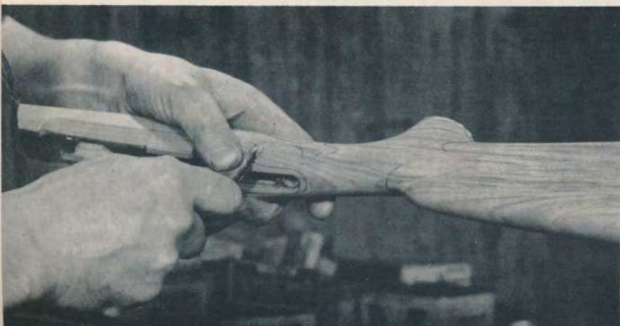
Biesen accurately inscribes a fleur-de-lis checkering pattern on the stock, then undercuts it carefully by hand. Biesen says that the result is checkering that doesn't look as if it had just been pasted on the gun.
