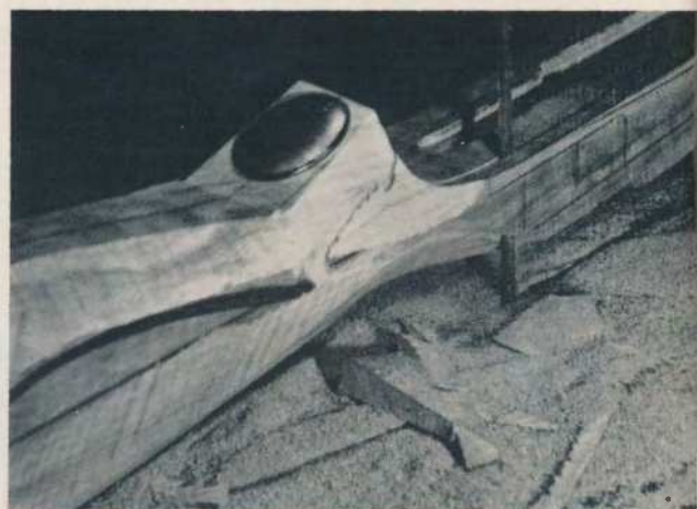
Using a band saw speeds the rough shaping operation. Note the pencil marks showing the position of the cheek piece and the layout of the action's depth in the stock.
