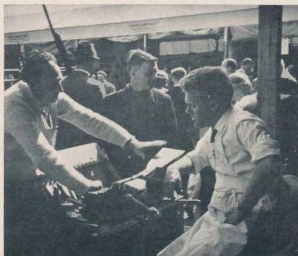
A Holland and Holland gunmaker demonstrates and discusses the problems of sidelock inletting.
