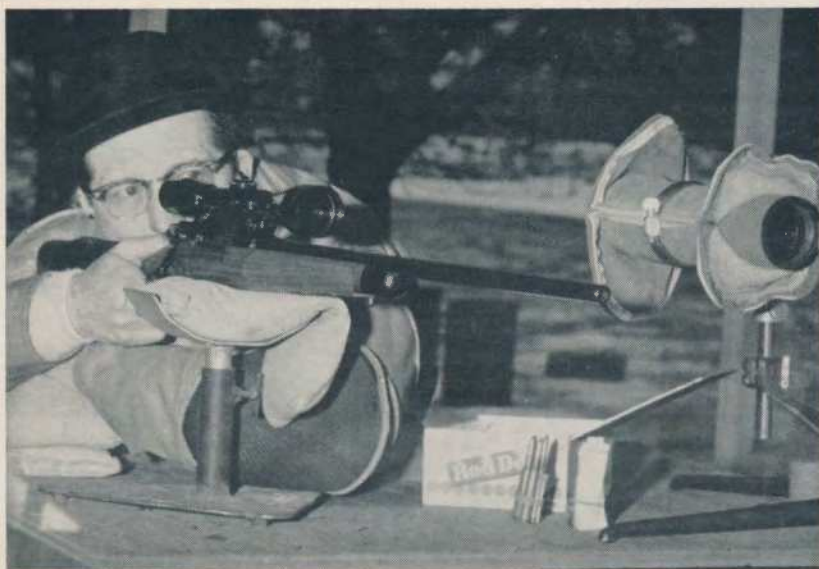
The crucial moment: range testing. Biesen always test fires any gun ordered from him for chamber tool marks and also runs a series of proof loads through the gun. However beautiful, it must shoot.
