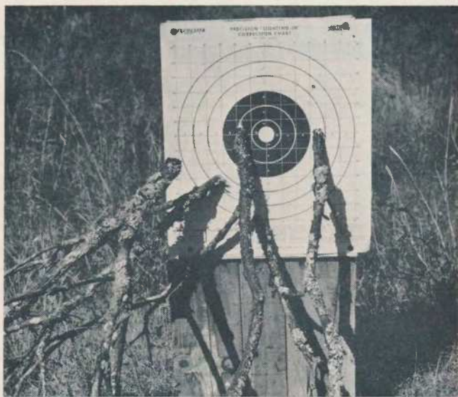
Above: Dead limbs will cause the greatest deflection. Below: Bullet pieces recovered show the destruction occurring when a branch is hit. Many were not found.
