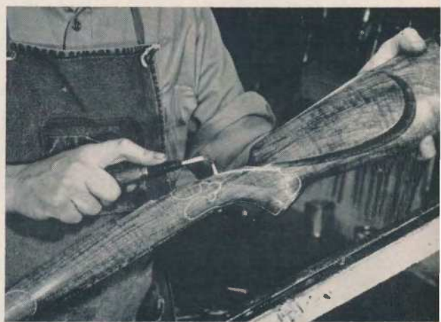
Beginning the 24 line per inch checkering, Biesen has already applied the epoxy finish. "Wet or dry" #400 and #600 grit are used to buff the finish between coats of the resin.
