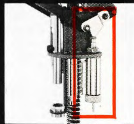
Cam-actuated reconditioning station
