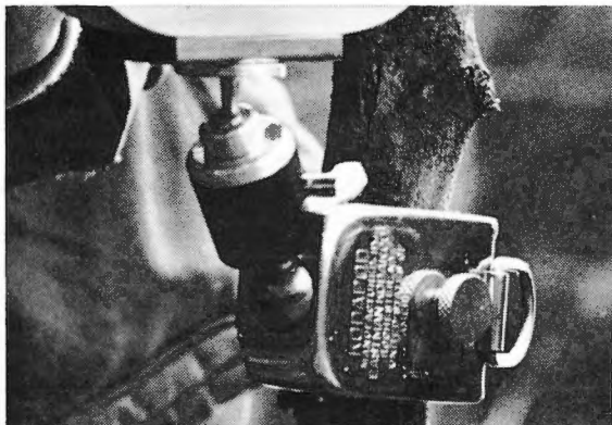
Simple fore-end rest attached to the tilt table and Kodapod will give you bench rest steadiness for increased accuracy on shots at long range.
