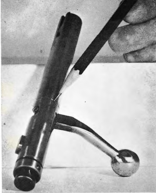
Pencil points to place where a thin shim washer can be placed to correct headspace.
