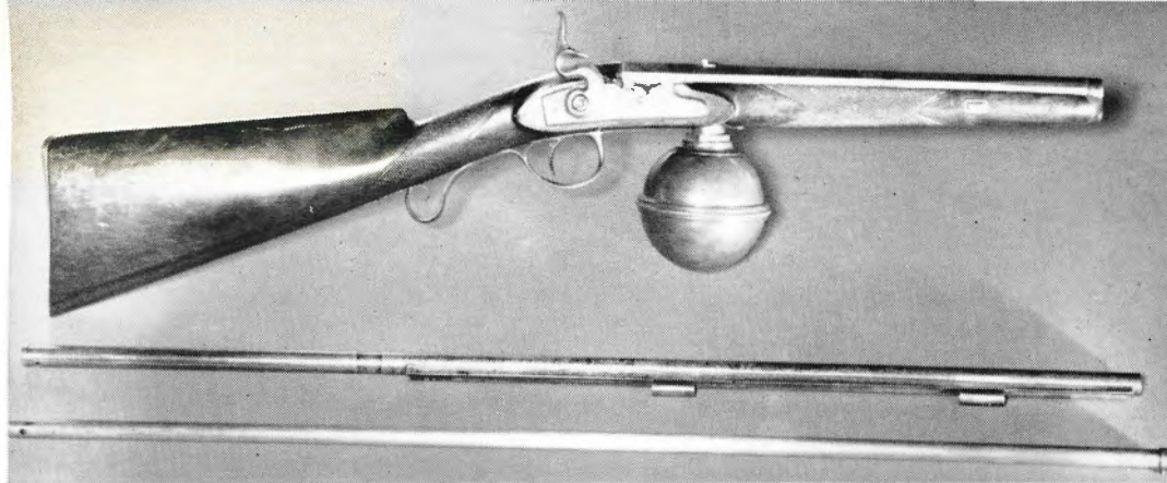
The unmarked air gun at left is only one of the three in this article that has action that is obviously faked. Gun is shown taken down (above) to show separate barrel liner.
