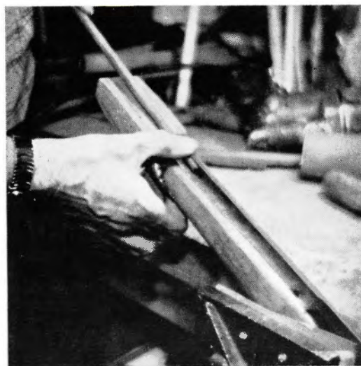
Illustrations show various steps taken in the installation of the fore-end tip. An array of good sharp rasps, round and flat, are essential, and so is a lot of patience.
