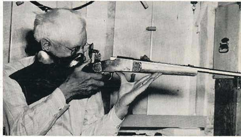
This .22 caliber Schuetzen target rifle by J. Hubel of Salzburg, Austria, has optical peep and D.S. triggers.
