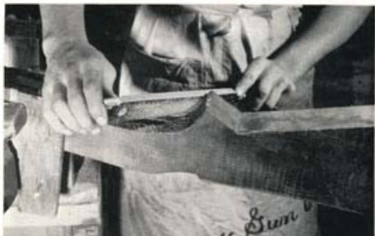
Holders include file (above), plane, and rocker or convex type to form all kinds of flat, curved shapes in hard wood.
