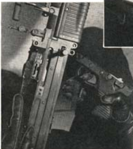
Firing pin in bolt is held back until gas operating rod closes action, locking bolt and then firing cap.
