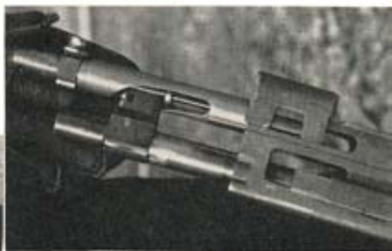
Firing pin in bolt is held back until gas operating rod closes action, locking bolt and then firing cap.
