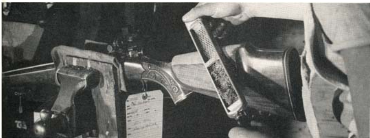
Set in file-type holder, Surform shreds off long curls of wood as if by many tiny blades, does not clog like wood rasp because teeth are open at back. Final comb height is shaped with Surform.
