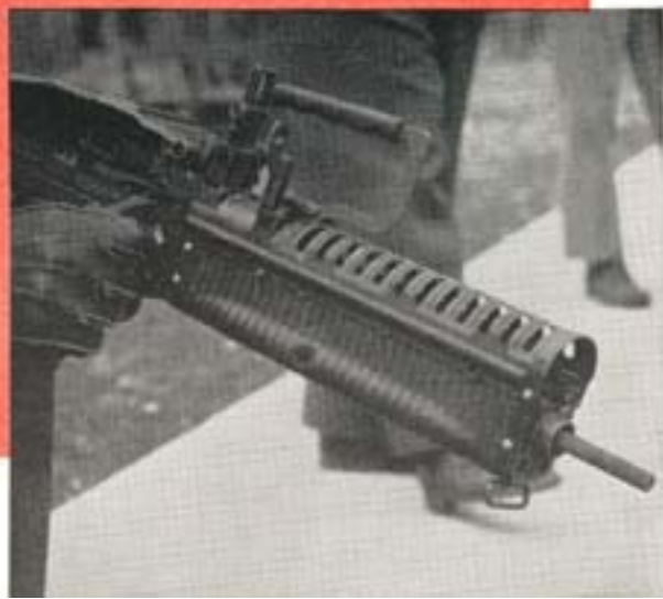
Flat clip by fingers holds grip pins in; cocking handle is shown with bolt open. At right, by handle, thumb piece lifts up to free barrel for quick removal in cleaning.
