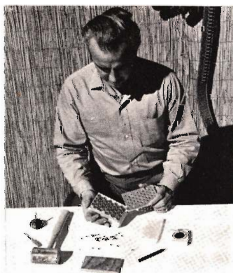
Bodrie uses loader of own invention to fill batch of unprimed hulls with wax pressed from block of paraffine. Next step is to ready primer plate on top of wax-loaded shells and manually insert caps. Inexpensive device is rapid loader for wax-bullet quick draw practice.
