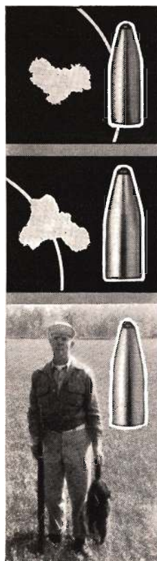
Five 22 cal. 60 gr. Hornady Bullets fired from a 22-250 varmint with Douglas standard barrel
