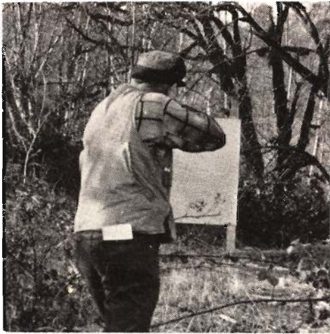
Sell's pattern board is steel sheet on 2 x 4s, daubed with white lead in motor oil. Patterns are brushed over for following shot.
