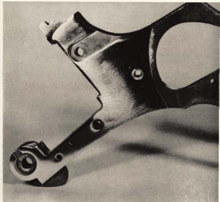
Incorrect polish of steel will result in graduated color on gun from blue-black (right) through straws to mud gray (left).
