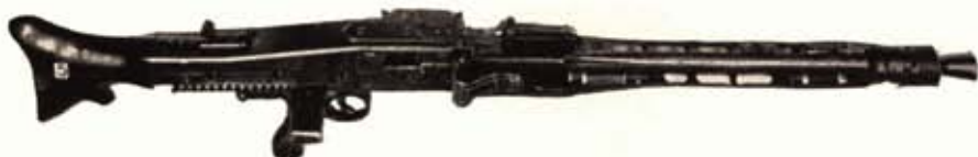
Original German MG 42 in 7.9 caliber was built for cheap production, weighed 25 pounds with steel construction, shot 1200 a minute, had one-second barrel change.
