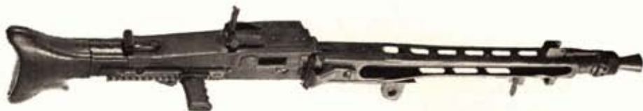
Unsuccessful U.S. copy of MG 42 did not allow for difference in case length to .30-06. Same feed was later used in light-alloy and plastic M60 gun which weighs 23 pounds.
