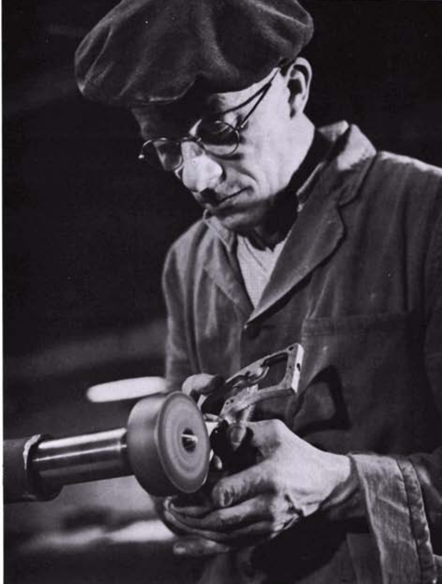
Half-dozen polishing wheels of many shapes and degrees of grit were used by Johnson preparing Webley to heat blue.
