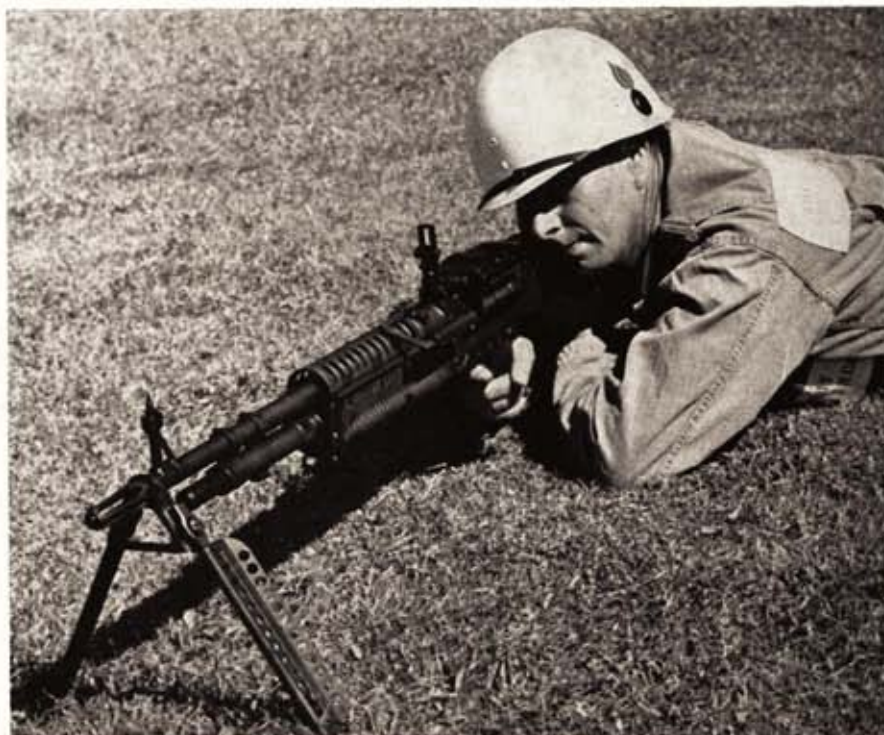
Army's new M60 machine gun is beefed-up combination of German FG-42 breech action plus belt feed like MG 42. Pivot lock at root of "U" handle frees barrel.
