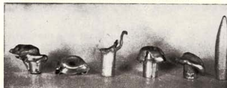
Remaining bullets in same order, after recovery, show Sierra slug (left) weighing 93 grains, Nosley (fourth from left) weighing 145 grains. Bullet at far right is unfired .30 caliber.
