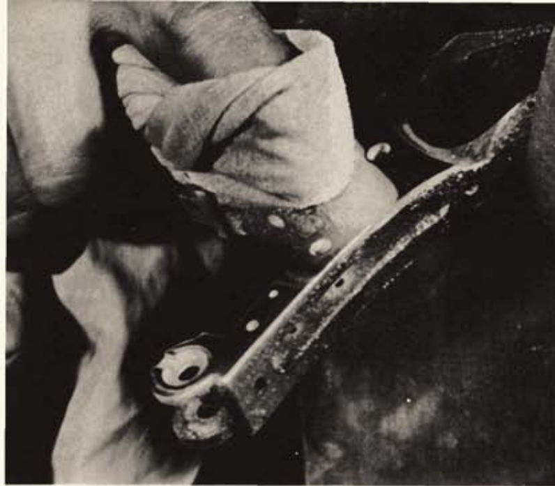
Perfect polish is essential on pistol frame to obtain perfect heat blue color. Work is often wiped with whiting on a rag.
