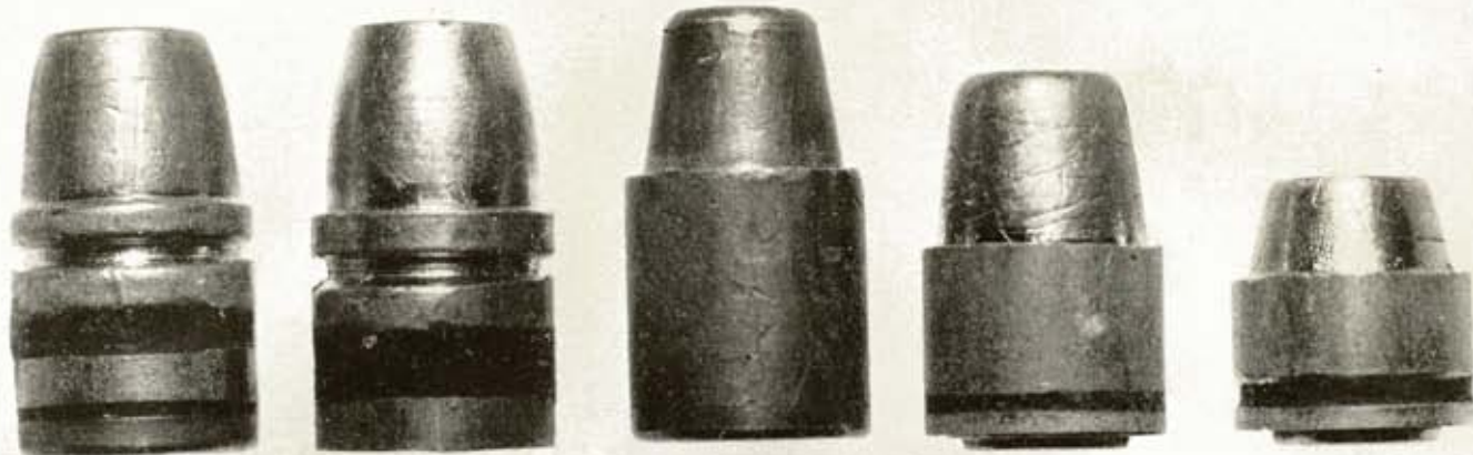
Bullets performing well in .44 Magnum handloads are: 235 grain Thompson gas check; 250 gr. Keith; 250 gr. Hollywood swaged; 220 gr. and 158 gr. Prot-X-bore. Latter can be loaded to 1700 feet per second, fastest in any .44.
