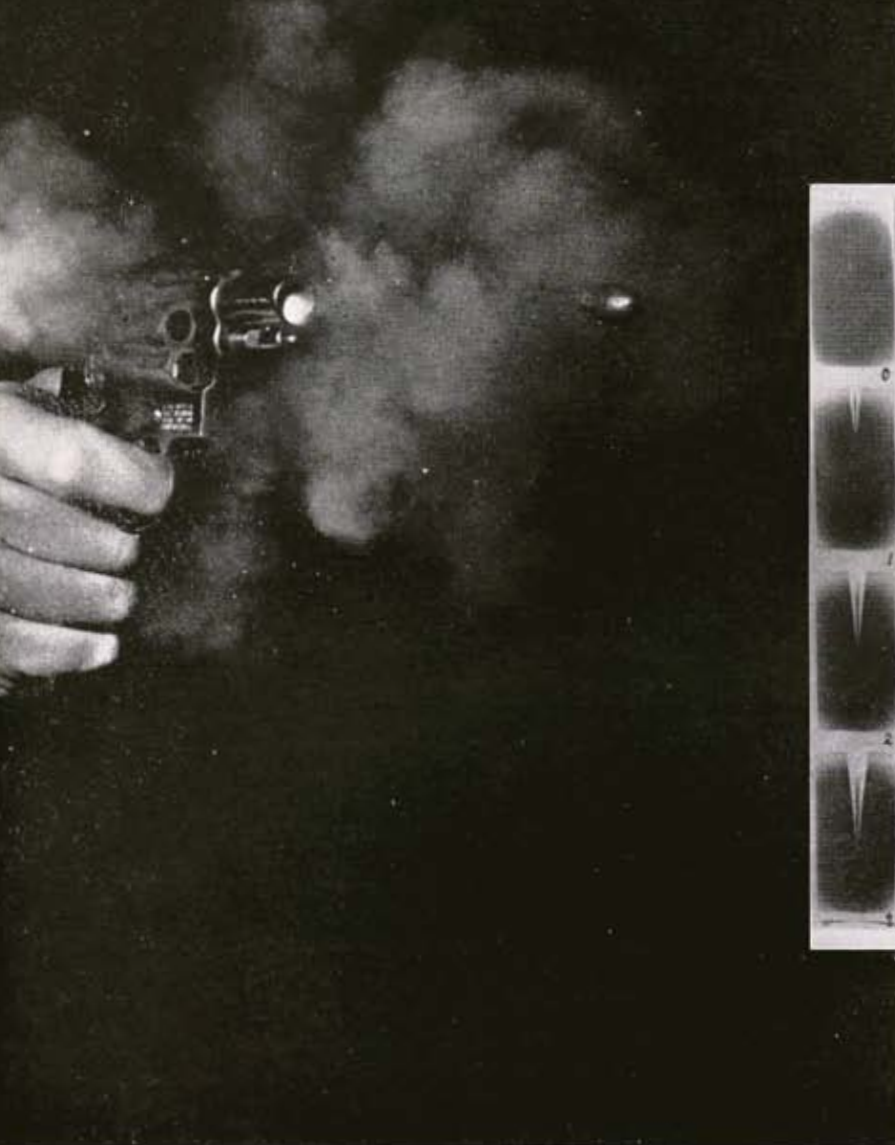
Movie of how wound is made was done by firing steel ball into water and observing how it made hole which changed size.
