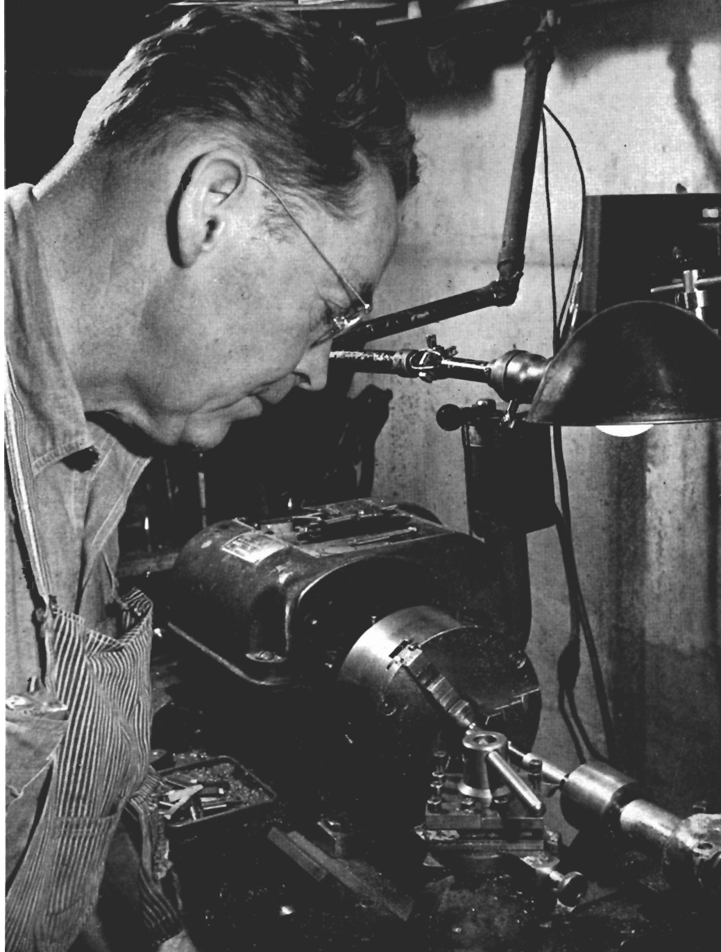
Chicago custom gunsmith George Pearsall works to close tolerances with his lathe in making cut which reduces body of Colt auto pistol barrel, avoiding unnecessary bushing friction in recoil, but leaves front end uncut.
