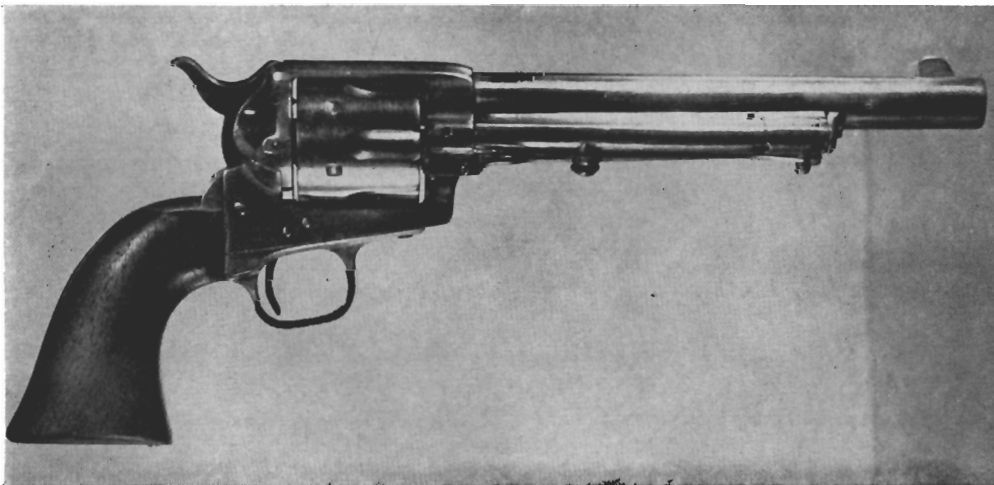
Slow reloading of SAA led to design of complicated ejector device which indexed cylinder, popped out shells. It was very unsuccessful in Army tests.
