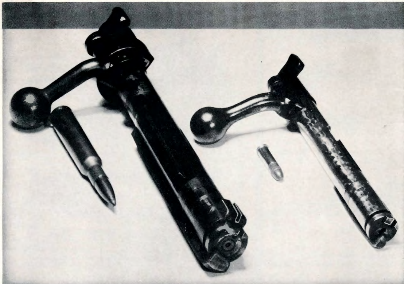
Note centered firing pin holes on full size bolt at left and .22 bolt at right.
