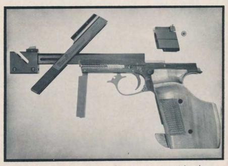
To clear the slide for cleaning, first remove rear sight, drop barrel weight, and ease slide back off frame and then forward.
