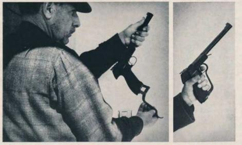
The Walther Model LP-2 air pistol is intended for match target shooting. With a weight of 46 oz., a barrel of  $9\frac{1}{2}$ ", and an overall of  $12\frac{3}{2}$ ", this pistol ain't meant for boys! It is a big gun and it takes some living with to hold it steady. Imported by Interarmco Ltd., the new LP-2 carries a price tag of \$72. For the handgunner who is determined to stay in best practice during the winter, this target number is worth its price.
