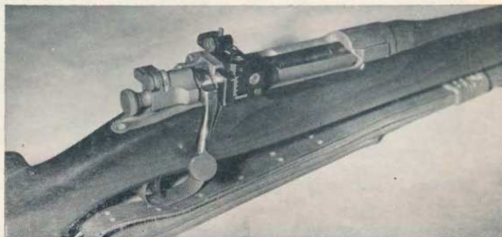
Above: Extension attaches easily with setscrews. Below: Reworked bolt fits saddle scabbard neatly.
