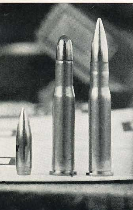
Loading on testing bench (above) saves time. A Sierra 168 grain boat-tail match bullet (left) is shown with a Remington factory load and one of author's handloads. At right, the 168 grain Sierra International bullet is seated in case.
