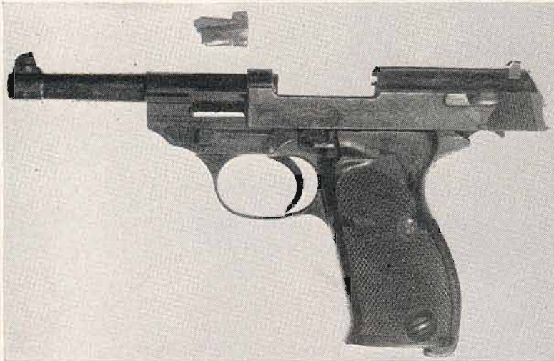
In P-38 phantom, locking block is shown in correct position, under barrel at slide and down in frame cut. X-ray permits study of inside design function.
