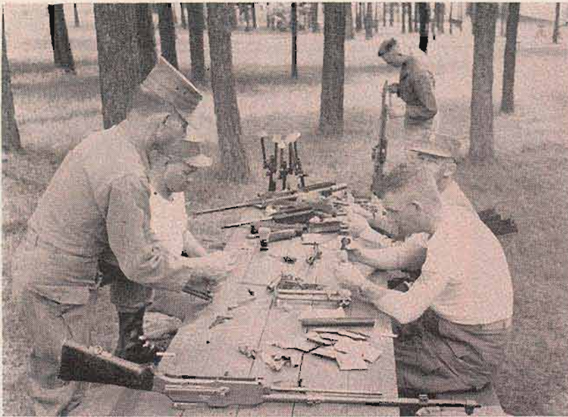
As Sgt. (left) bears down on roll pin to strip B.A.R. gas adjust plug, tattooed AR-man whisks off dust from sight leaf using shaving brush.
