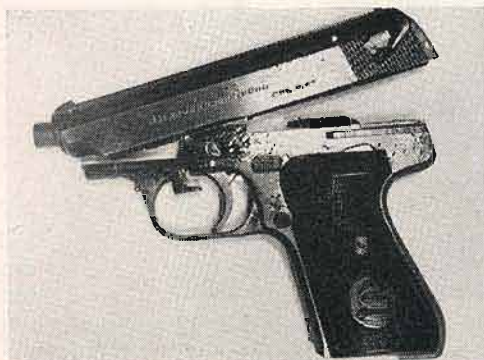
Sauer DA38 was giving trouble in ejecting. Gunsmiths fiddled with it but shadowgraph revealed that recoil spring was bent on barrel.
