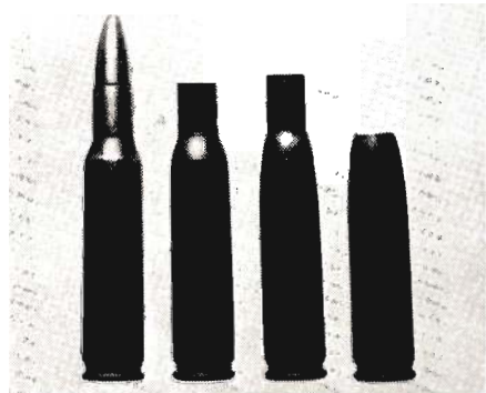
Good .222 reload compared with cases stretched in die without lubrication.
