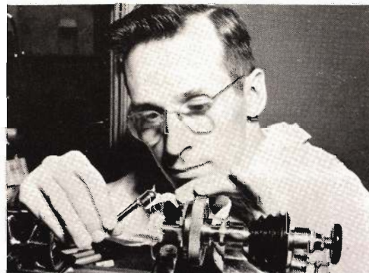
Jeweler's lathe was needed to make screws and drill holes in model guns; also does polishing.
