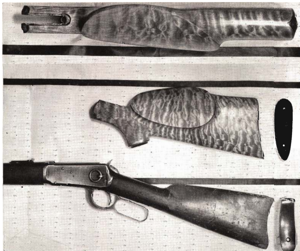
Guymon light rifle (left) has wide forearm for recoil control, with cheek piece sloped to allow gun to kick away from cheek. Same design is in Hi-Wall maple stock (above) which has plate sloped to reduce torque on firing. Old M94 carbine was notorious kicker.
