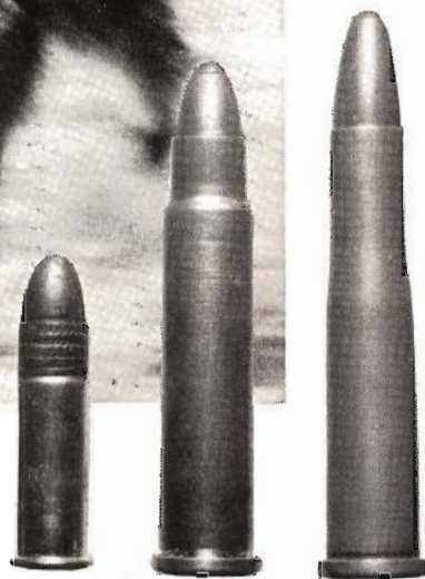
Novel handgun varmint round, ideal for wary coyotes, is Kay-Chuk (center) contrasted with .22 LR, and Hornet (rt.) from which it is made.
