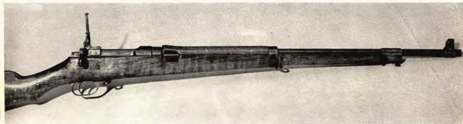
Mark II** has longer barrel (30 1/2" instead of 26 1/2") and sight fixed permanently to receiver, may be target issue.
