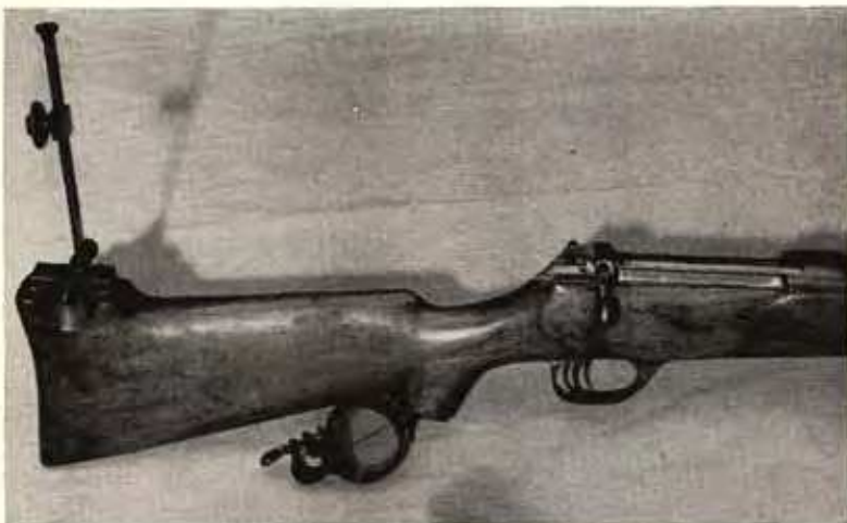
Rear sight on stock heel and glass plate foresight were fitted to .300 H & H Magnum target rifle. Arm was used for fine accuracy at 1000 yard's range. Shooter lay prone on back, held gun over feet.
