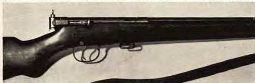
Unique Ross .22 straight-pull trainer was announced in 1911 catalog. It operated like the regular .303 and was locked by a trigger-operated bolt safety.
