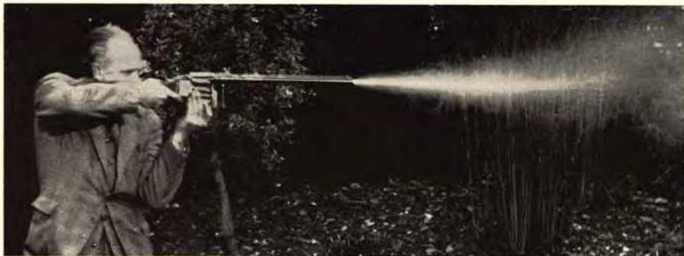
Firing Treeby gun is author, noted arms expert. Lever below barrel holds it tightly on chamber front slope, avoids gas leakage, giving more power.
