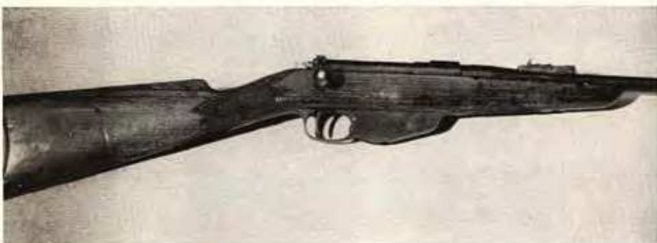
Rear sight on stock heel and glass plate foresight were fitted to .300 H & H Magnum target rifle. Arm was used for fine accuracy at 1000 yard's range. Shooter lay prone on back, held gun over feet.
