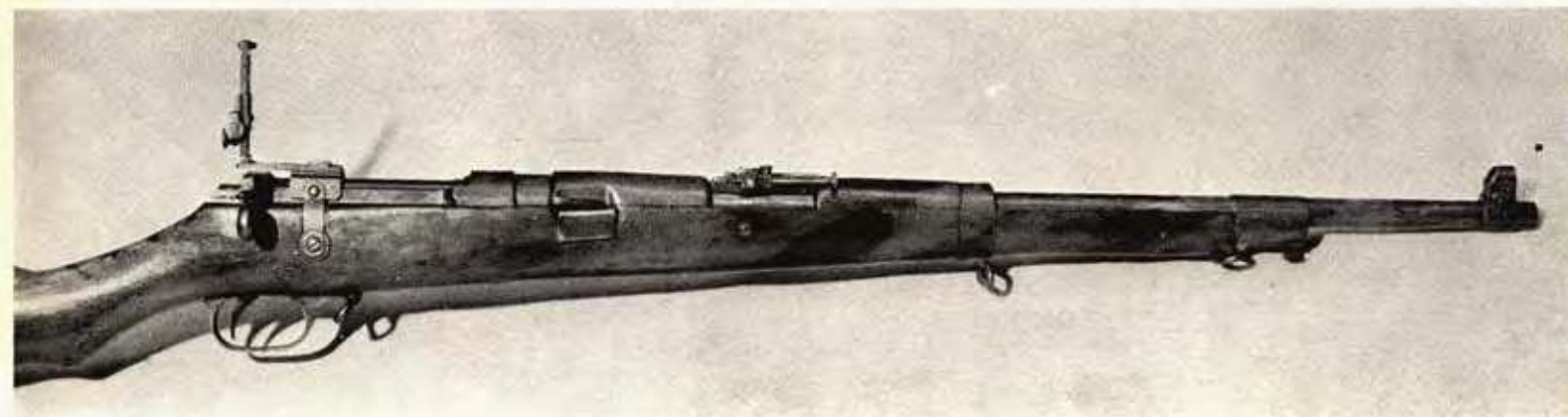
Modified Mark II** is sometimes called "1st sniper model," with accessory rear sight that is attached using stock bolt.
