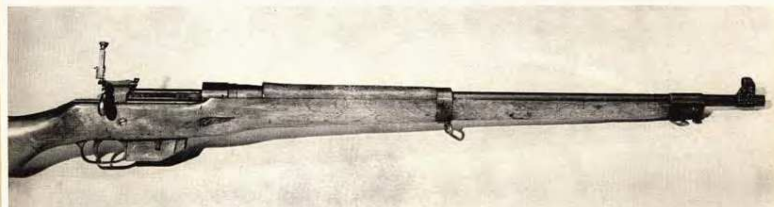
Model 1910 Mk III is common Canadian service rifle, has multiple lug bolt head that can be assembled unsafely.
