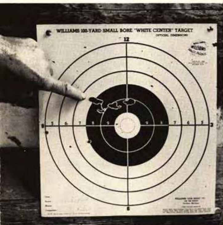
Even heavy bullets keyhole at too high velocity and, once tumbling, will deflect badly if they hit a twig.
