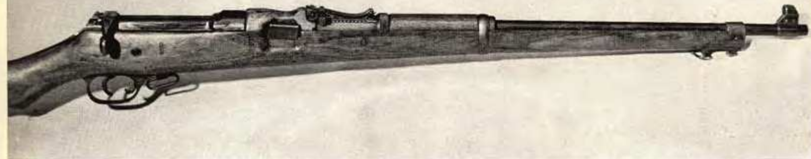
Early Mark II* (1905) military had magazine lever; was fitted with tangent curve rear sight for caliber .303.
