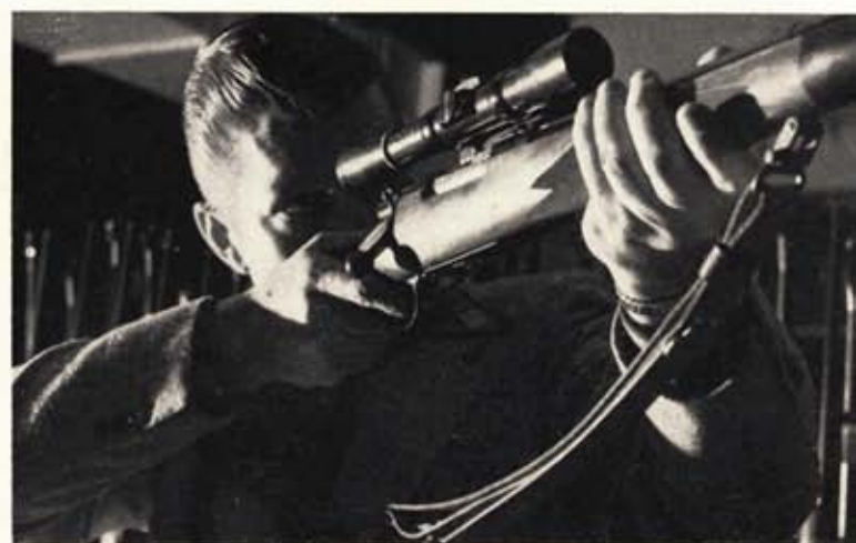
Scope should have bright, crisp image; be placed so eye naturally takes sight as rifle is brought in line.
