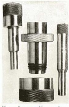
Harvey die set assembles around core and gas check which are then swaged.
