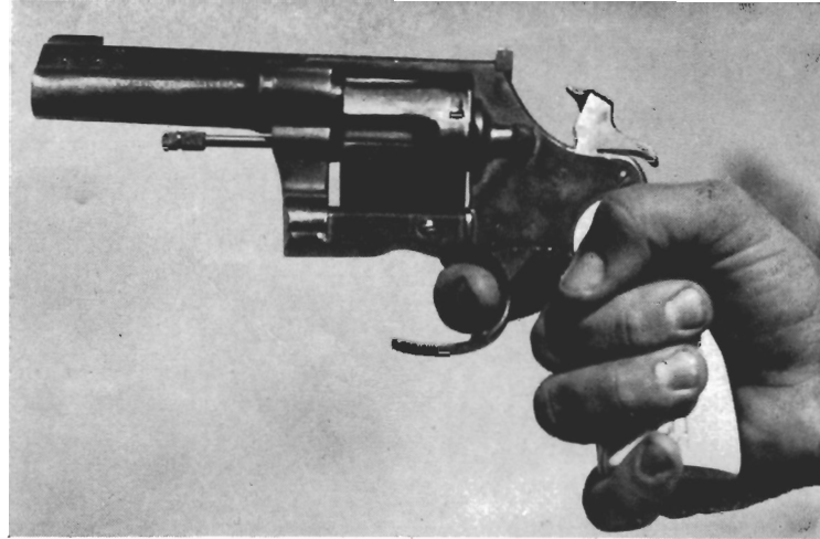
Colt New Service in .357 Magnum makes fine belly gun with guard cut away and sighting rib added.
