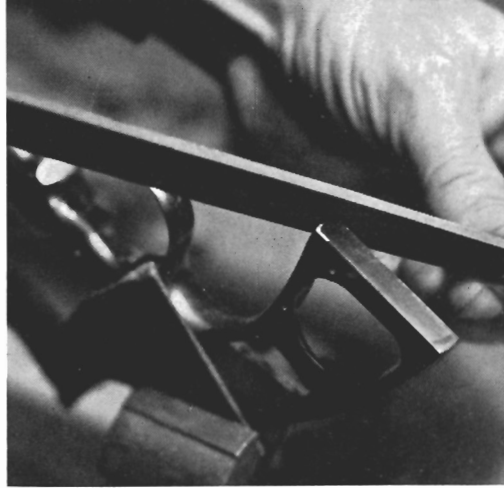
Sharp corners of butt frame should be cut off and rounded with a file. This reduces bulk of gun in shoulder holster under coat.
