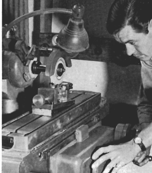
Frame bottom against which guard strap must fit closely is finished smooth by machinist using angled jig on a precision grinder.
