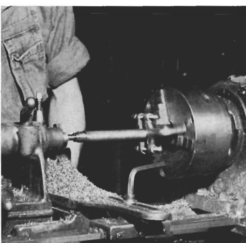
Barrel blank is "turned" or tapered for shape on lathe. Next step is threading of barrel for mounting on the work frame.
