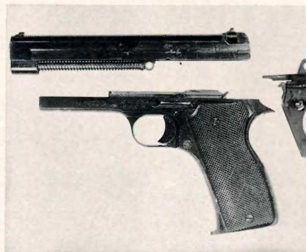
The M-1935A field strips like the Colt .45 Auto except that the firing assembly strips as a subassembly.
