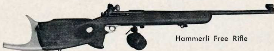
Armors from the U.S. Army Marksmanship Training Unit at Ft. Benning used a Remington Model 40X barreled action to make up this free rifle.
