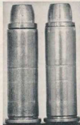
Crimp seat die adjusted for normal length case (right) will not crimp bullet in a short case properly.
