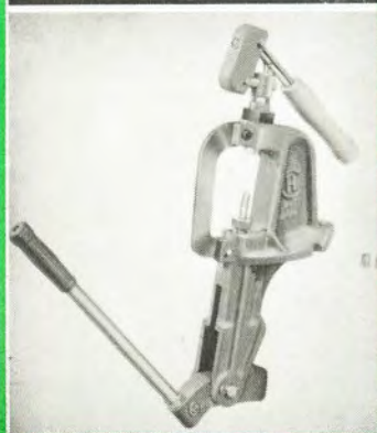
Top, the C-H Swag-O-Matic is a speedy and highly efficient bullet swaging unit. Below, C press with brace, ejector.
