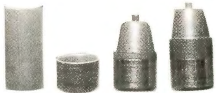
Carefully cut core, half jacket, and bullets with nose bleed-offs. Adjustments of the dies are critical.
