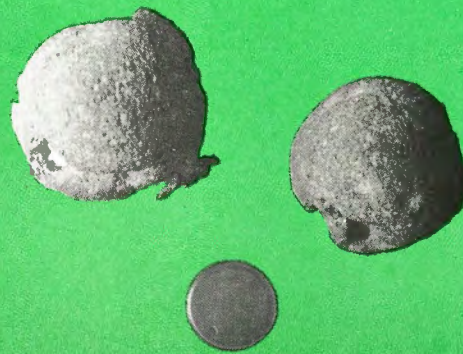
Soft bullet shows maximum slugging with hot load. At right, two .44 Mag., bullets, gas check factory bullet left, swaged right.
