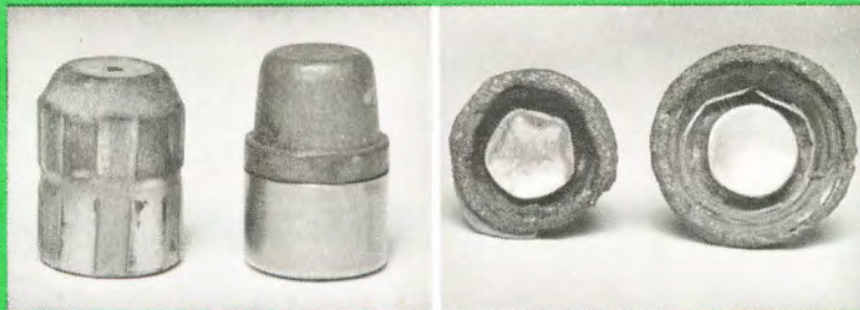
Soft bullet shows maximum slugging with hot load. At right, two .44 Mag., bullets, gas check factory bullet left, swaged right.
