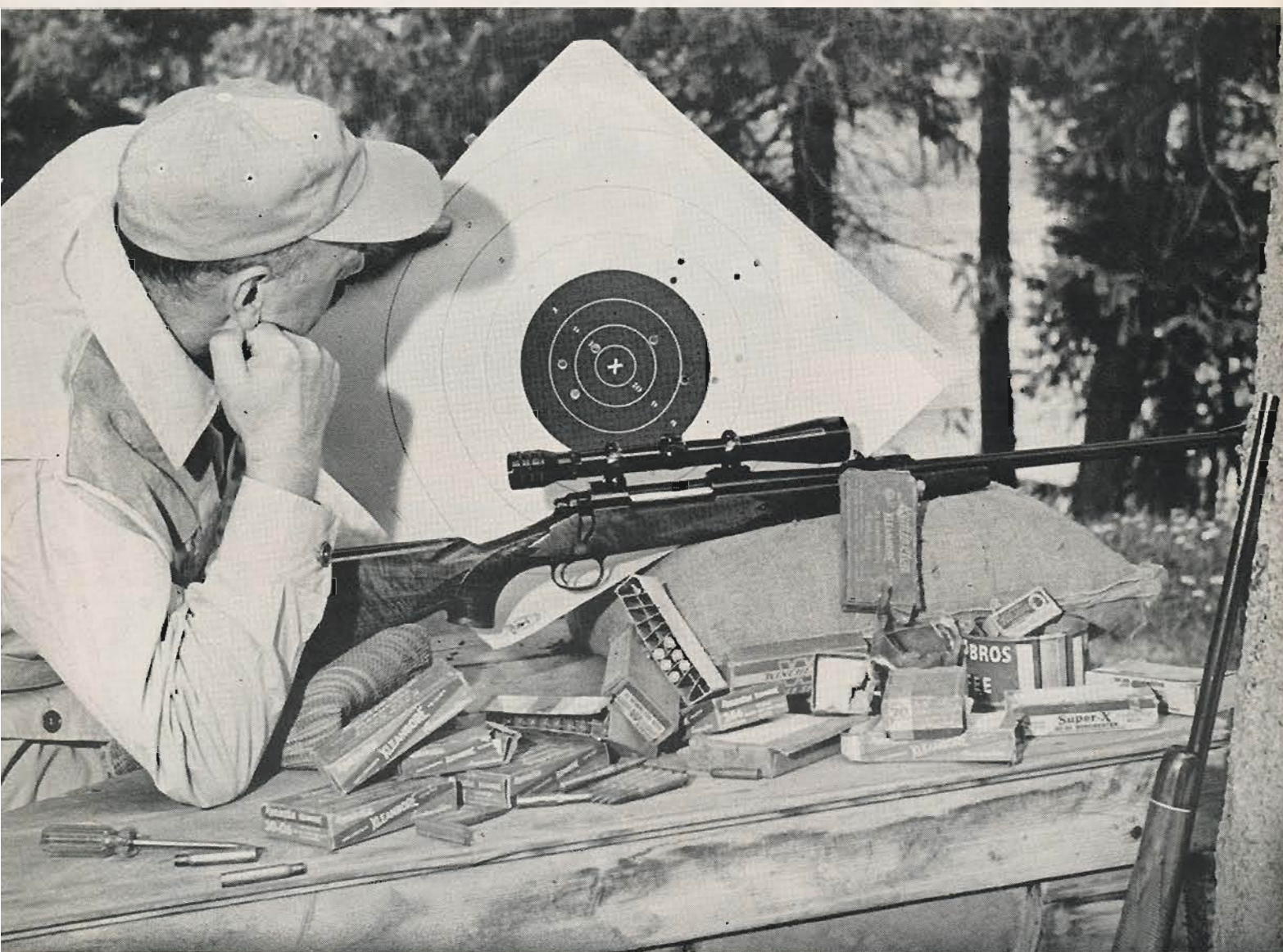
The author studies one of the targets fired in elaborate "mixed ammo" tests. Rifle is a Remington Model 700, in 7 mm Magnum. Target shows wide spacing of groups from two different bullet weights in both 7 mm and .30-06 calibers.
