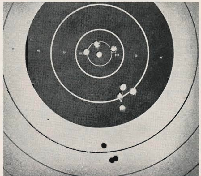
Three types of factory .30-30 ammunition, from 94 Winchester at 50 yards, gave point of impact span that could cause a miss on game at 100 yard range.
