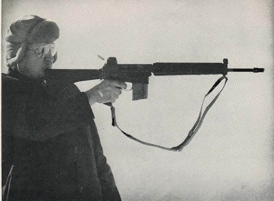
Extremely light recoil of the AR-18 is demonstrated by shooter who holds rifle to his chin with one hand while firing full-automatic. Note empties in the air.
