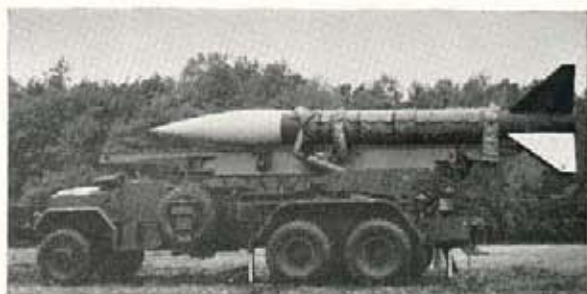
Current U.S. Army tactical missile is the solid propellant "Honest John" now with NATO forces.
