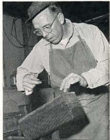
Wire basket is used for component parts of each gun to avoid mix-up, assure good bluing of small parts.
