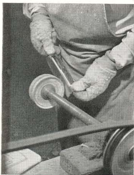
Quality of bluing job depends on care metal gets before bluing. All rust, old bluing must be removed.
