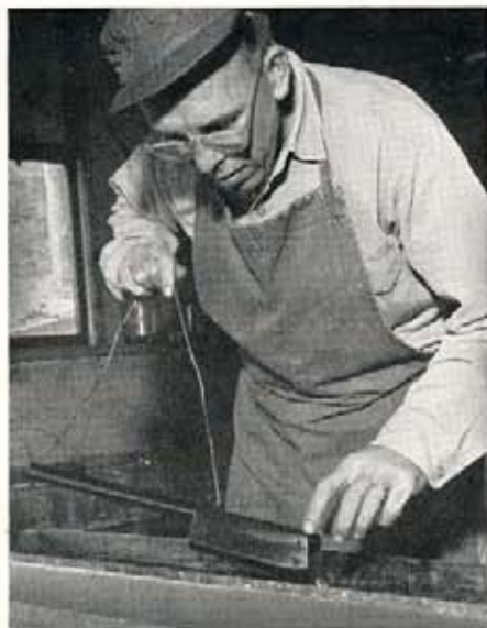
Large pieces are suspended on wire hangers in tank. Exact temperature control is vital to perfect bluing.
