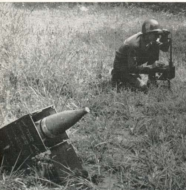
French ENTAC is one man unit, and missile is directed via control box en route to target.
