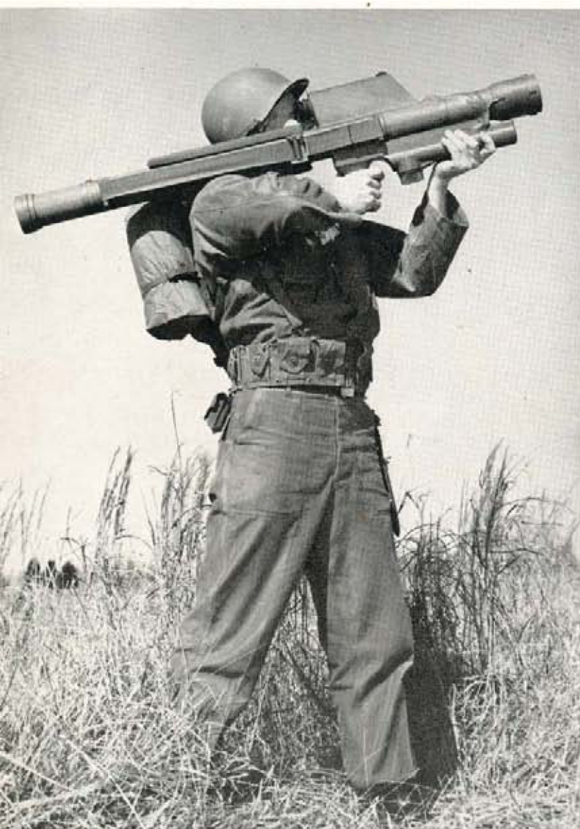
"Redeye" is G.I.'s defense against low-flying planes. It is guided by infra-red system, carries high-explosive head.
