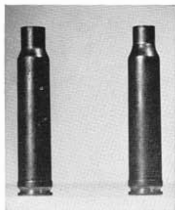
Griffin & Howe M70 was Newton-chambered for author, recorded 3165 f.p.s. Rt., short .338 is re-formed to Newton chamber (right case). Bullets are Hornady, Speer, Nosler, and gas check.
