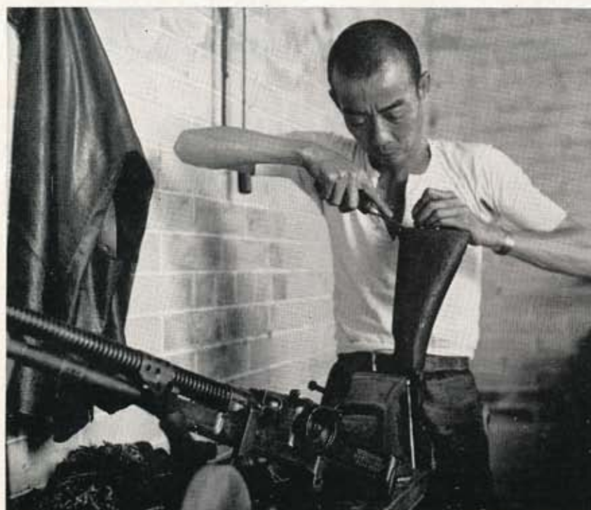
Armorer fits new butt stock, inlets end for old plate to be attached. Gun is Czech Brno 8 mm light machine gun. Some CZ guns were made in China.
