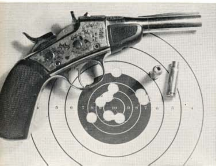
Favorite "turtle gun" is .401 Special Remington on light rolling block action. Big bullets print accurately with moderate loads. Right, .25 K-Hornet Jr. Ruger, extensively tested in return-to-battery rest on author's basement range, firing over thousand shots in barrel-load studies.
