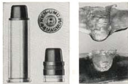
Factory .44 Mag swaged GC bullet makes smaller hole than (top) Jugular.
