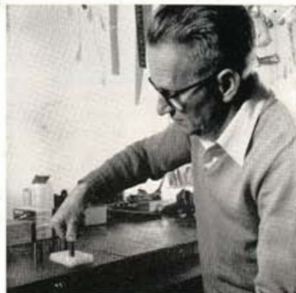
Pushing unprimed case into Parawax, Shaffer then seats normal primer in regular tool. Case has flash hole drilled out, should be kept separate from cases for full loads.
