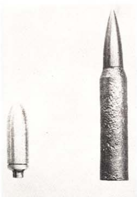
Light aluminum bullet and combustible 8mm fit various CETME rifles. In center, Walther caseless 9mm may be model for new Russ rocket cannon.
