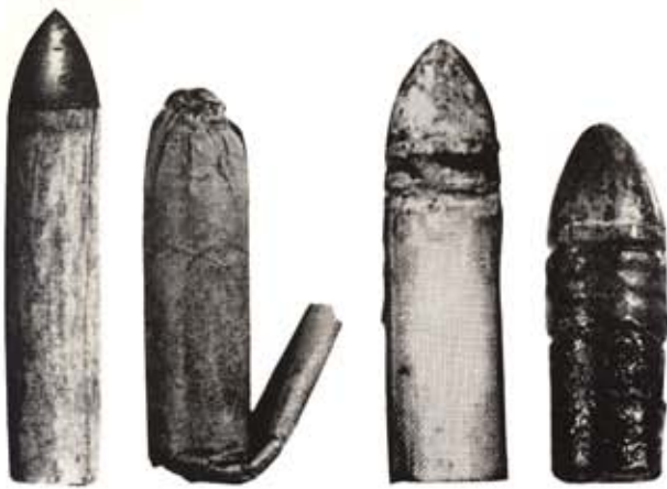
Civil War caseless cartridges used in muzzle- and early breech-loaders did not seal chamber; guns often had weird mechanisms to do this. Cases were of (l-to-r) tinfoil, paper tied with string, linen and shellaced silk.
