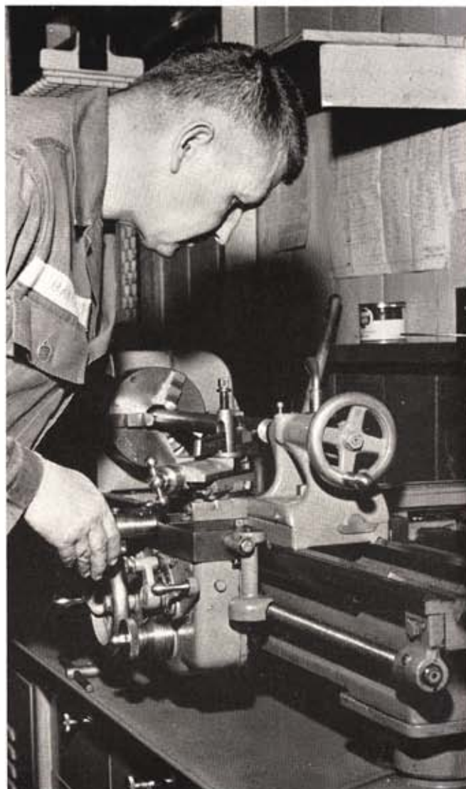
Complete gunsmithing is done in Unit shop. M/Sgt. Glenn Baker here turns barrel ready for action fitting. Glass bedding of service M1 rifles is also done by armorers.
