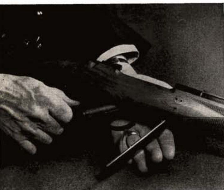
Hinged floorplate of Rigby Mauser magazine permits dropping soft nosed rounds, loading with solids, while still covering wild animal with shell in the chamber of weapon.
