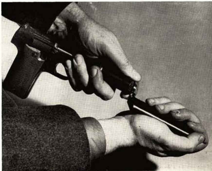
Magnificently engraved Kersten-bolted AYA O/U is only "2nd grade" gun of major Eibar gun factory. Single trigger is U.S. importer design. Below, clip spur handily helps release takedown muzzle collar on popular 9 mm Astra pistol.
