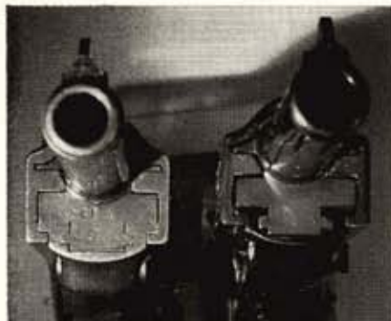
Old P-38 shows closer slide - barrel fitting but new guns (right) shoot well.
