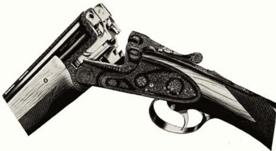
Magnificently engraved Kersten-bolted AYA O/U is only "2nd grade" gun of major Eibar gun factory. Single trigger is U.S. importer design. Below, clip spur handily helps release takedown muzzle collar on popular 9 mm Astra pistol.
