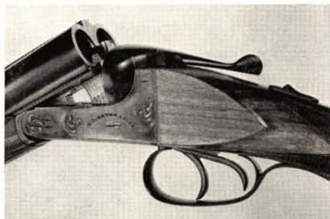
Stöcker Sauer by famous German maker shows shallow receiver associated with doubles where tubes lie sideways.
