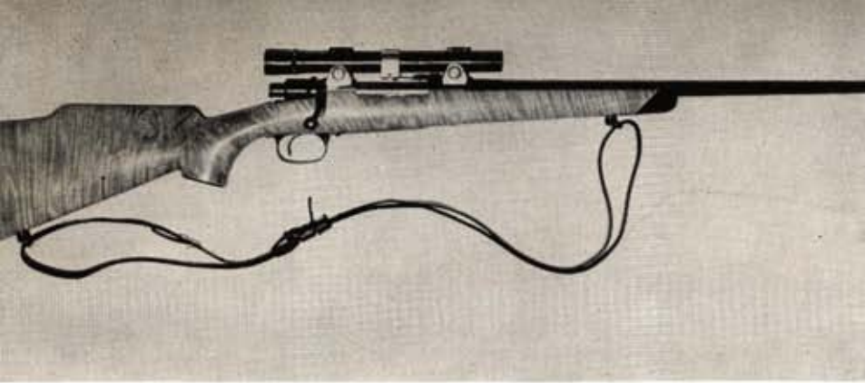
Custom-built 8 mm on trimmed '98 Mauser action weighs under 6 lbs. with sling. Scope is 2 1/2X Leupold.
