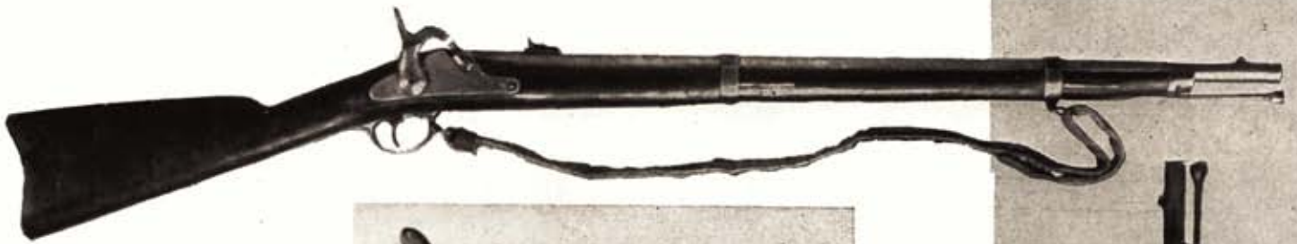
Richmond musketoon made by tools from Harpers Ferry Arsenal used unfinished salvage U.S. lock blanks forged for Maynard tape primer (right.)
