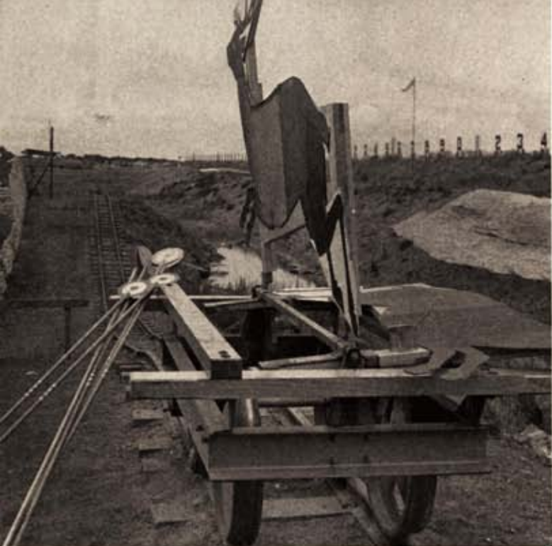
Running deer target mounted on rail dolly flashes across Olympic competitors' line of sight in about four seconds.
