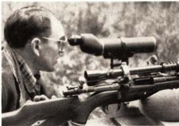
Crow-shooter sights in Mauser with .22-250 premium Pfeifer barrel and Unertl 12X scope from bench rest.
