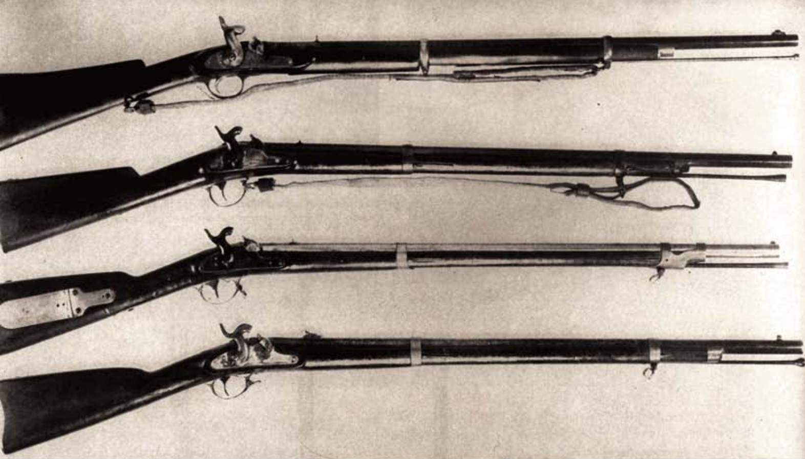
Cook rifle copies Enfield (top); J. P. Murray and Palmetto rifles (2nd & 3rd) were styled like U.S. M1841; Fayetteville rifle (bottom) used Harpers Ferry parts.
