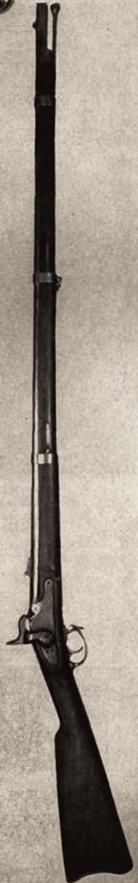
Richmond rifle was assembled from Harpers Ferry blank lock and captured U.S. 1863 barrel.
