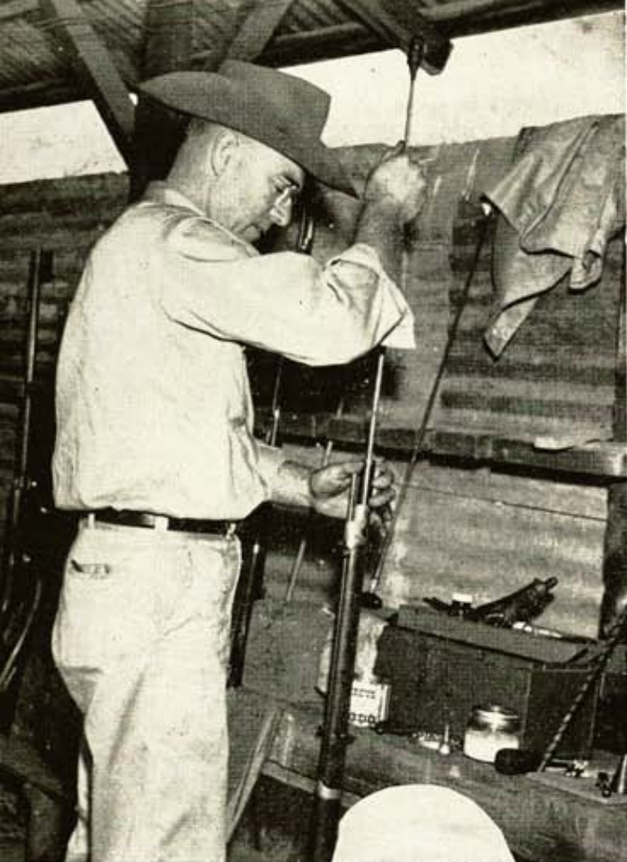
Swabbing bore between shots from M1842 rifle, J. P. Kraig of Compton, Calif., cleans powder fouling, helps accuracy.
