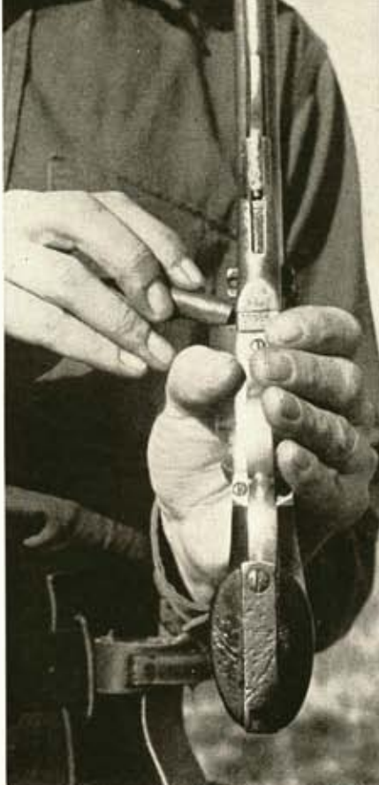
Measured charge is poured into each chamber with hammer on half-cock.
