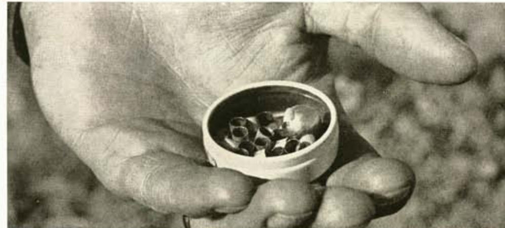
Small copper cups filled with mercury fulminate when struck by the hammer ignite the charges in chambers through individual tubes called "nipples."
