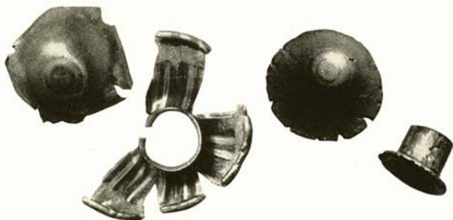
German service 9mm bullet shed its jacket (left) in penetrating \frac{1}{8} " steel plate but .45 slug burst jacket, flattened out and stopped cold (right) on steel.
