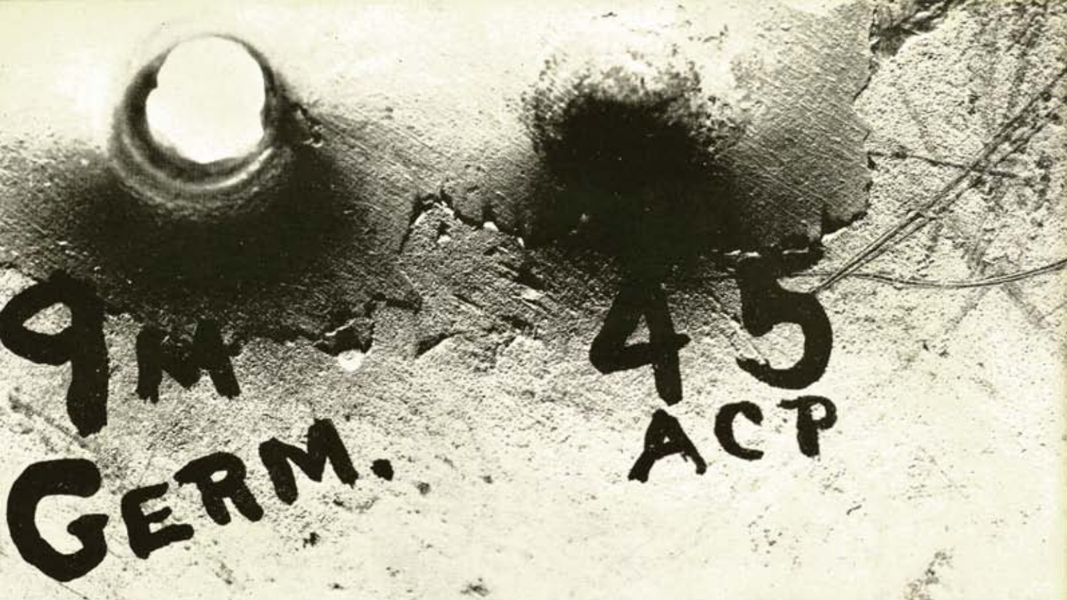
Heavy \frac{1}{8} " steel plate fired at in tests reveals comparative power of U.S. .45 cartridge and German service bullet.
