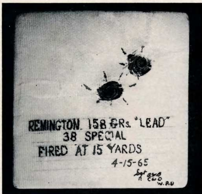
A single 1/8 inch thick Doron fiber glass panel will stop bullets traveling at velocities up to 1100 fps.
