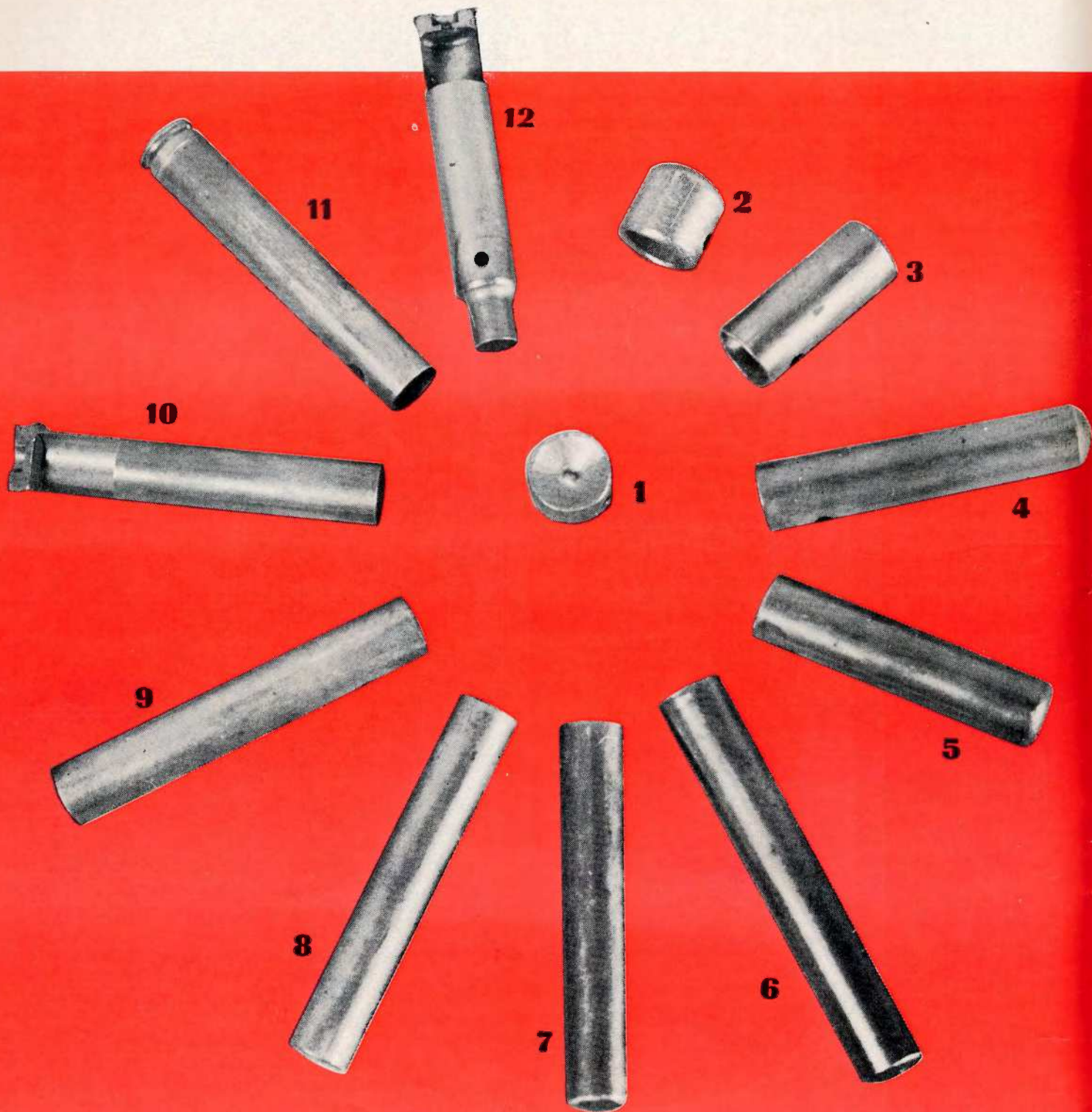
Beginning with the double concave slug in the center Speer used eleven draw steps in producing cases. This series is for a .300 Weatherby Magnum case.
