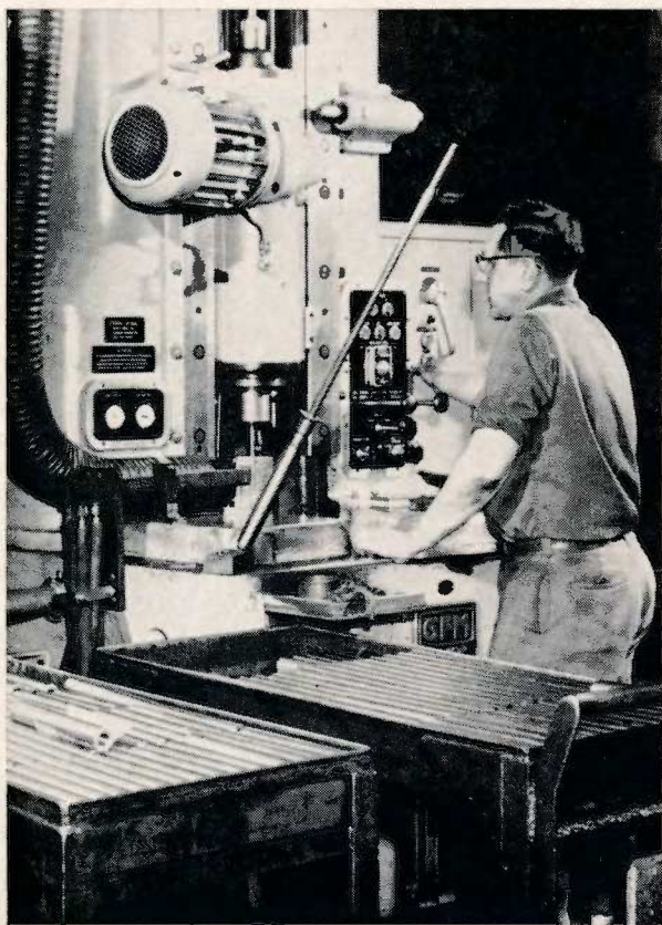
Above: Weatherby's barrel machine can forge in rifling. Left: Ithaca's similar machine forges shotgun barrels.
