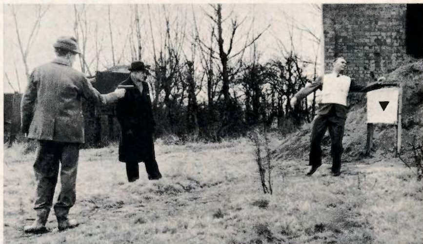
During tests the Wilkinson vest stopped bullets from a 9 mm Browning.
