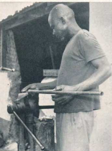
Barrels are made of steering rods taken from junked cars.
