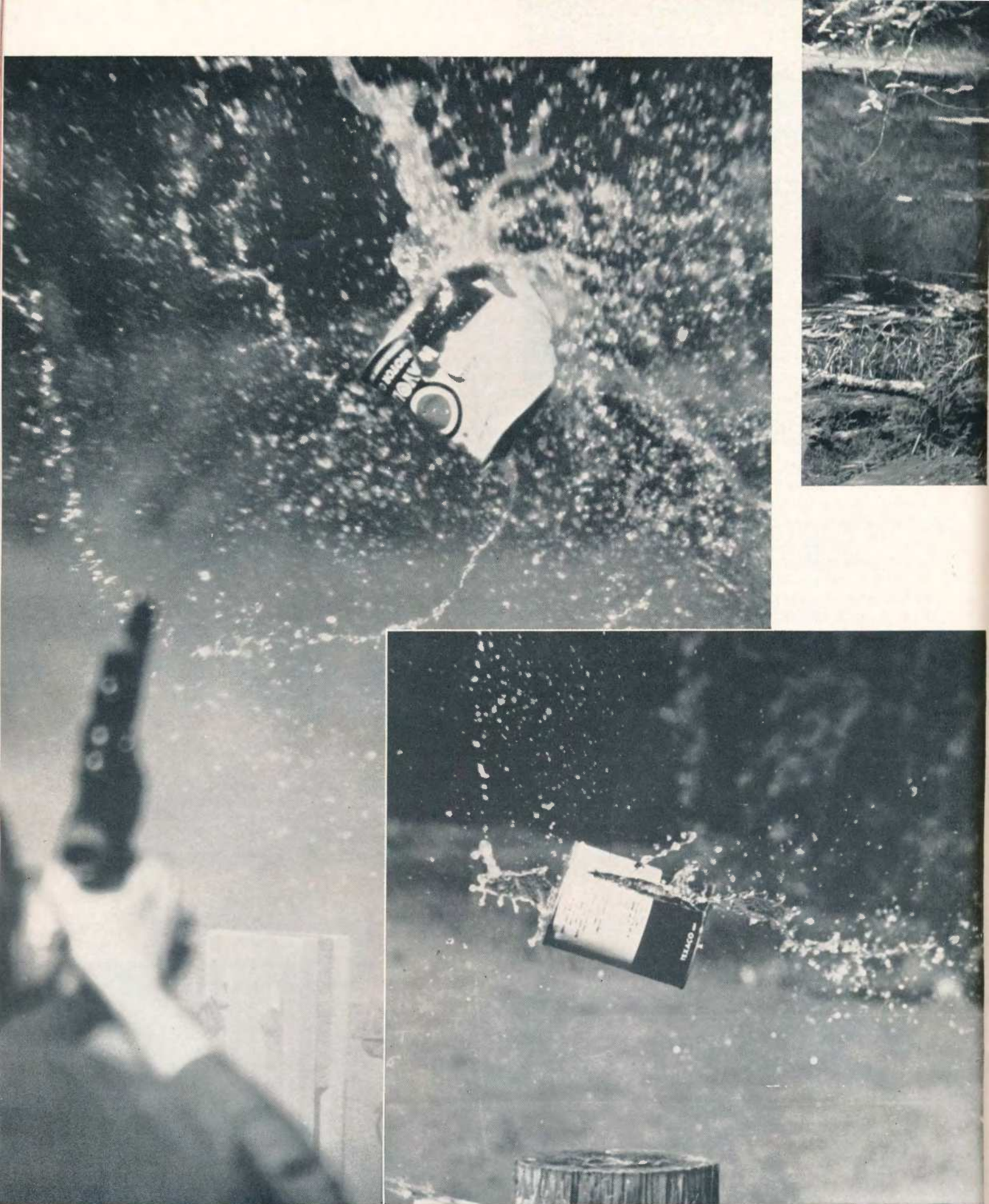
A cast 240 gr. semi-wadcutter from the .44 Magnum at 1430 fps thoroughly demolishes a quart can of water, while the .22 High Speed Hollow Point bullet only splits the seam of its water-filled can.
