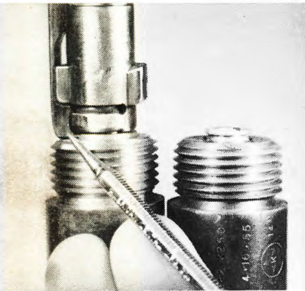
Left: Extractor fits into barrel slot; bolt face and stud shroud .444 rim. Normal case protrusion shown at right. Right: Bottom view, showing altered edge of bolt shroud.
