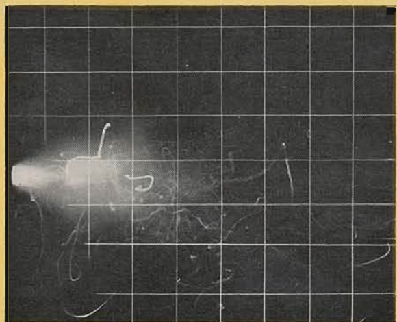
An open shutter photograph of the primer flash of a CCI Magnum #450 small rifle size primer.
