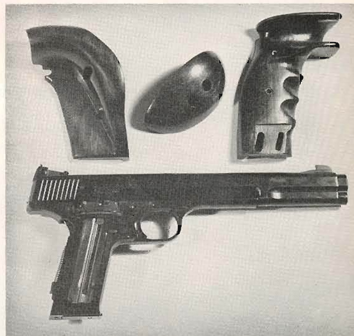
Photo above shows how palm rest is attached to right grip panel with two Allen head bolts and square nuts. Below are the three parts of the grips; finger grooves, checkering are optional.
