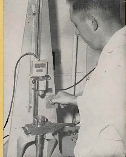
The Tinius-Olson drop tester, in use at Cascade Cartridge Company, shown (left) with the cartridge holder in the open position. At right, the ball of known weight is ready to be released and dropped onto the firing pin.
