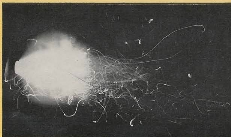
Flash of a CCI Magnum #250 primer shows the hot incendiary particles penetrating to ignite the entire powder charge.
