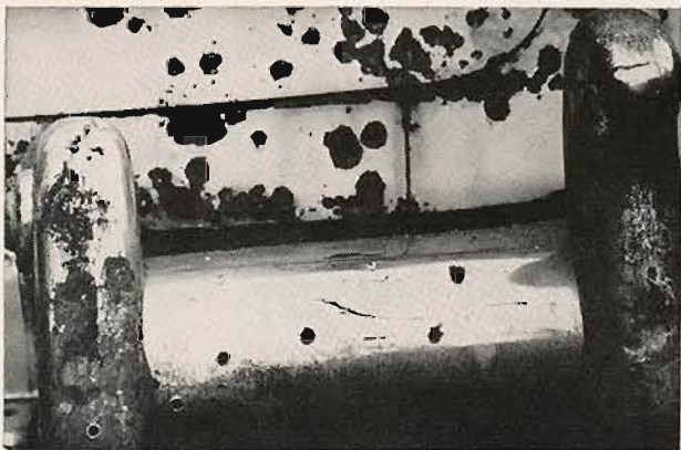
The 5.56 mm bullet of the AR-15 goes clear through the car bumper and it does not upset on contact.
