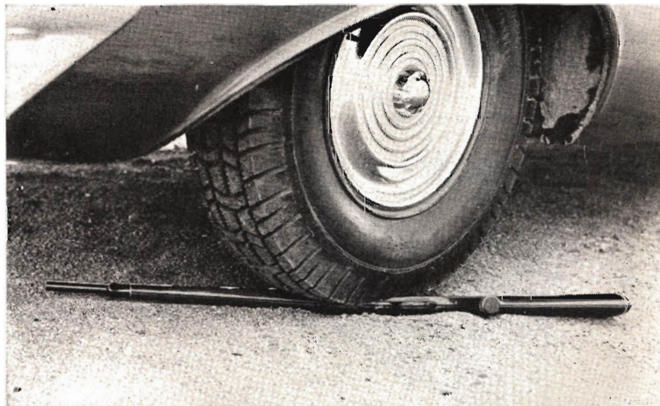
Impact and flexural strength of nylon-receiver rifle is proved by drastic smash-up tests. Gun was not smashed up in these tests.
