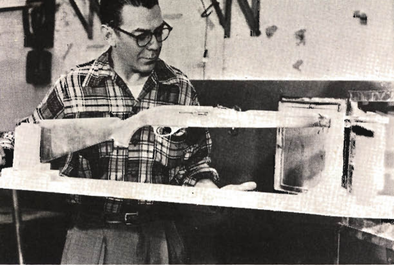
Choked with sawdust which would have gummed firearm made of usual materials, self-lubricating nylon gun fired OK.
