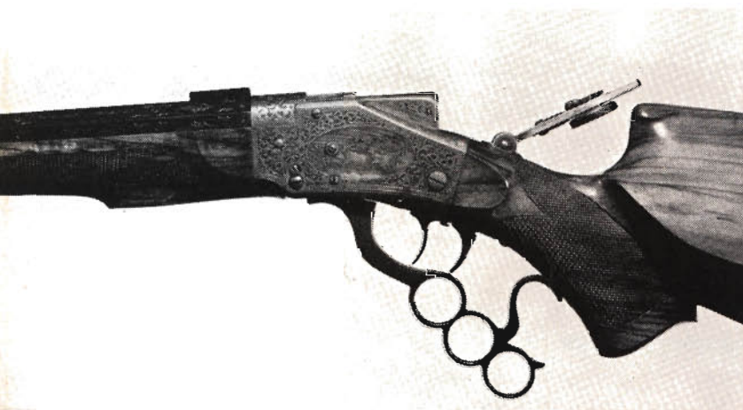
Borchardt action finished and beautifully engraved by gun-maker Schoyen of Denver is .38-55 caliber. Below, Sharps in Philadelphia made few rifles on actions of cap lock pistols.
