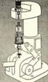
HOLLYWOOD "SENIOR" RELOADING TOOL set up for swaging bullets.
