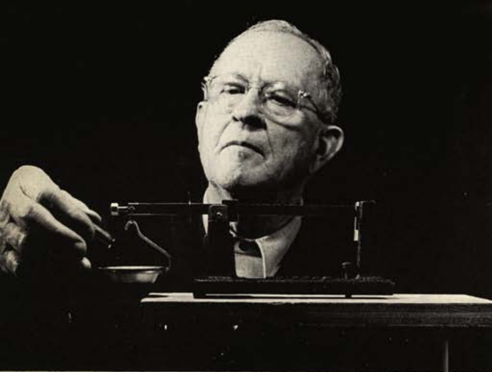
Handloading-bench refinements by Mears include scale board seated on peg to convenient eye-level.
