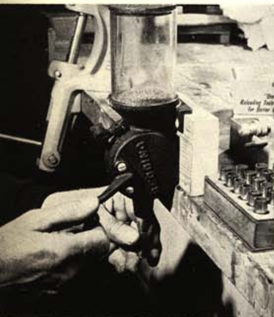
Powder measure is screwed to peg block that fits in holes drilled in bench.
