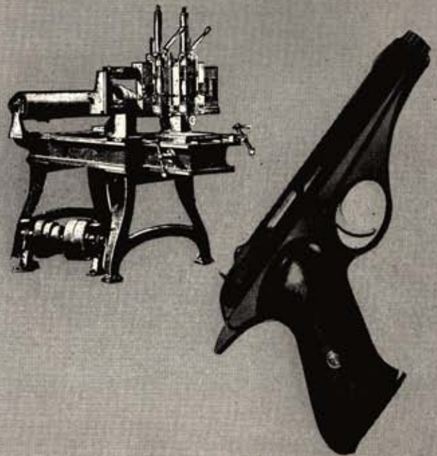
Basic tool for making muskets to modern pistols is double-spindle profiler, shown above cutting Marlin rifle frame. Current machine is identical with ones sold by Pratt & Whitney during last century.
