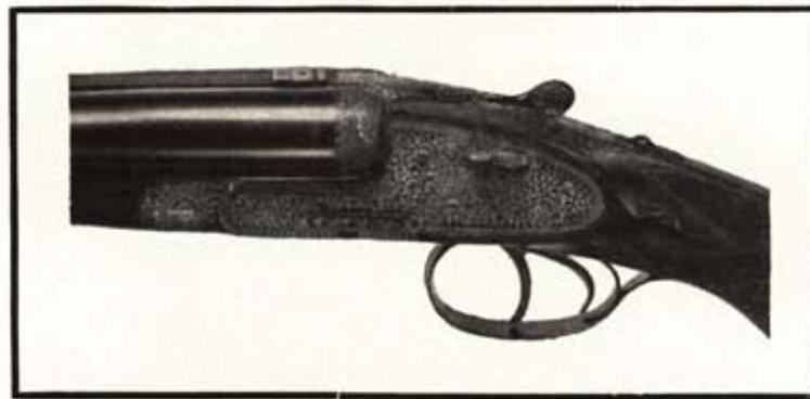
A & D box lock action like Webley double (top) from Abercrombie & Fitch and older Ithaca side-by (middle) take less stock fitting than Holland side-locks (bottom).
