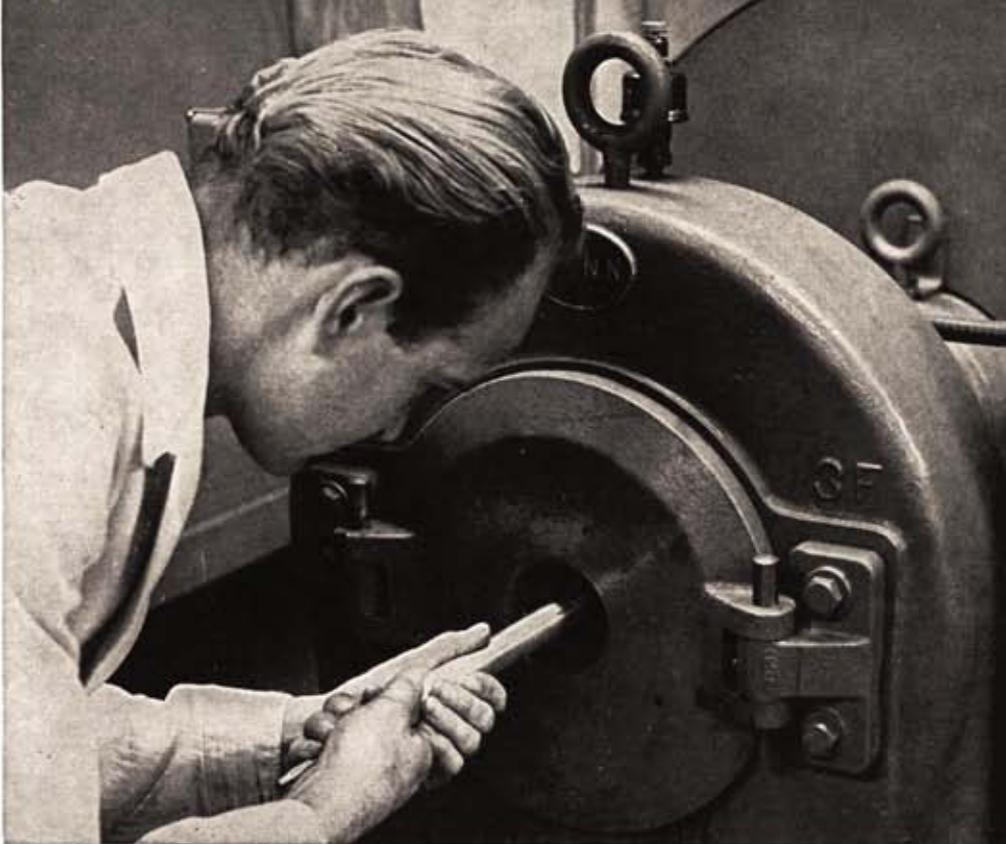
Swaging machine forms aluminum barrel jacket over stainless steel liner in fast operation for low-cost construction of erosion-resistant AR-10 barrels.
