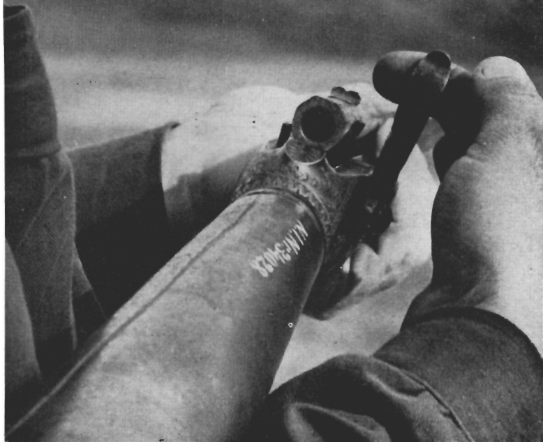
Cock is pulled to make gun ready for firing. Pulling trigger snaps cock, opening air chamber to fire rifle.
