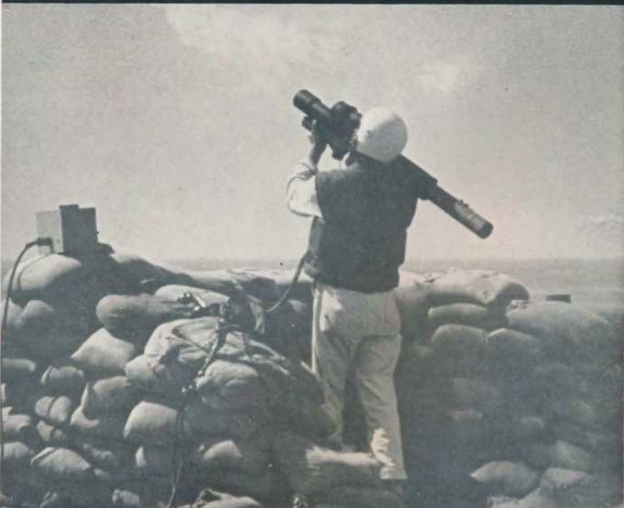
First stage of Redeye missile launches it from the tube. Second stage fires at a safe distance from gunner as it locks on target.
