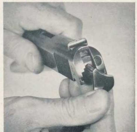
A Pressing firing pin clear, safety lock can then slide the stop out.
