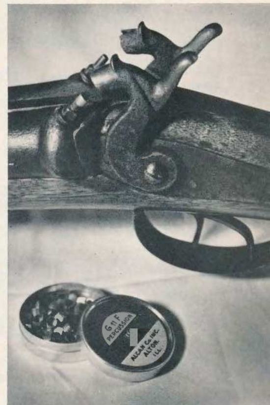
The proper size percussion cap will fit snugly onto the nipple neck.
