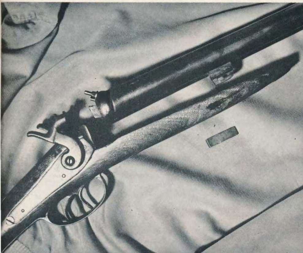
Barrel and stock are separated by knocking out the small wedge which binds the barrel lug to the stock. This is usually an easy process.
